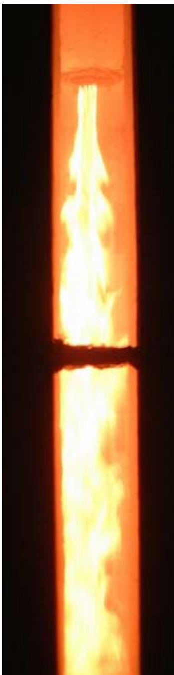
Figure 4. Stable Attached Coal Flame 17% Transport Air Oxygen, 900°C Walls
