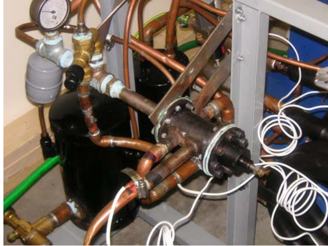
Figure 20. Closer View of the Ejector Device
