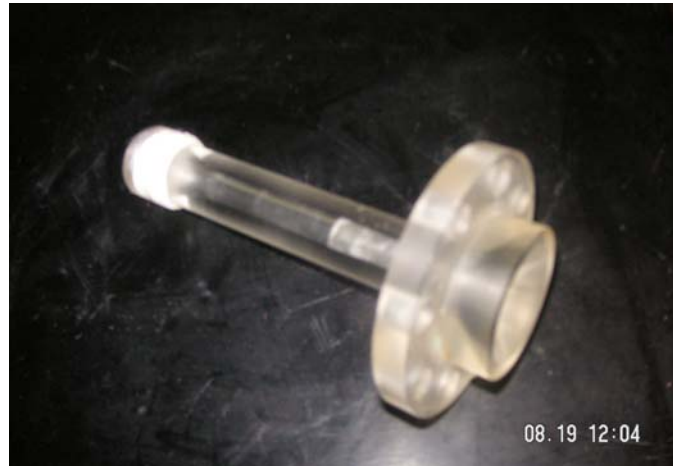
Figure 8. Ejector fabricated of transparent material for observing air-water mixture flow.
