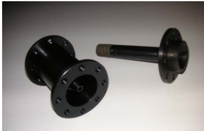
Figure 6. Two main components of the vapor-liquid ejector: housing with motive nozzle and vapor inlet (left) and ejector with mixing chamber and diffuser
