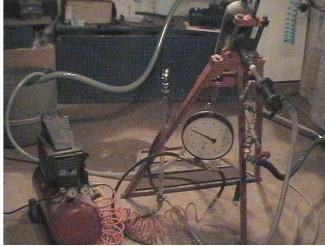
Figure 12. Nozzle (4) with transparent ejector (5) installed on the stand. Also, shows the compressor (8), rotameter (9) and pressure gauges p_4 (on the compressor) and p_5 (large). On the back visible open tank (7) and pump (10).
