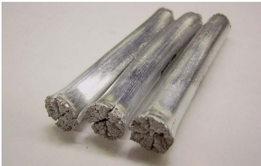
Figure 8: Consolidated rod from aluminum powder after extrusion.
