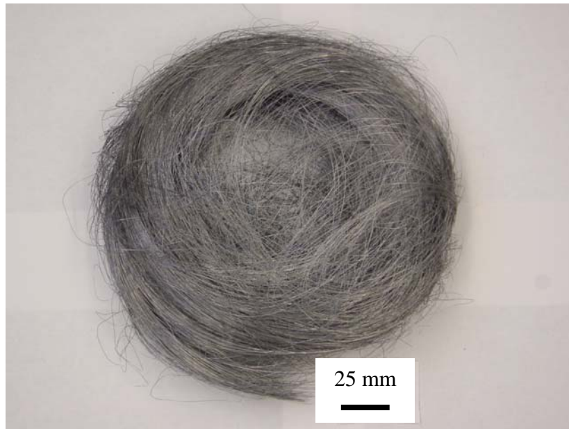
Figure 3: Cleaned scrap wire from industrial processing.
