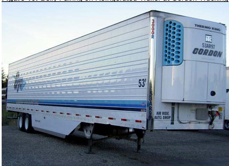
Figure 10: Belly Fairing on Refrigerated Trailer at Gordon Trucking
