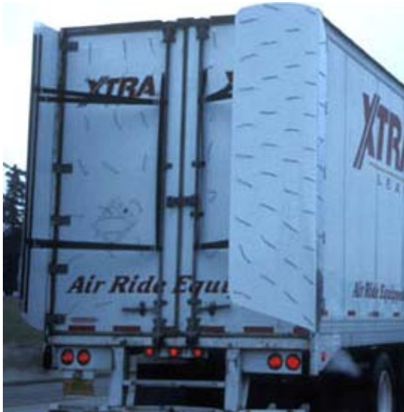
Figure 5: Initial road test vehicle with rear fairing Tuft strings enabled engineers to visualize air flow.
