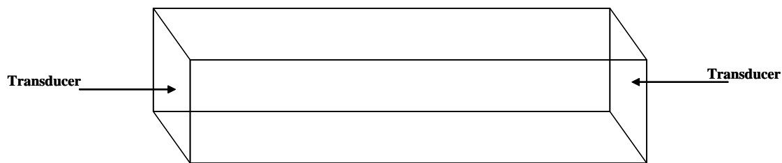
Figure 8. Ultrasonic measurement location and direction on tensile and Charpy impact specimen blanks.
