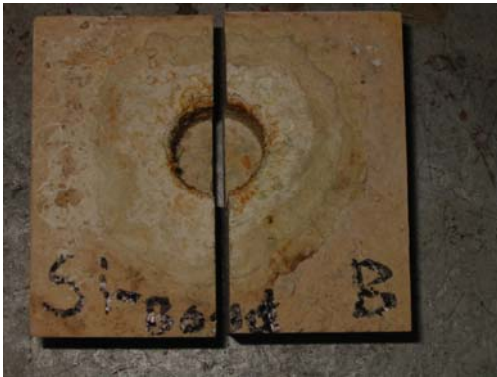
Fig. 1: A refractory cup in corrosion test.
