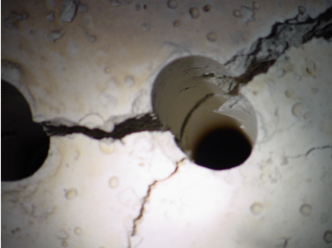
Figure 3 Enlargement showing critical delamination failure at 5-6" in depth and accompanying transverse cracking.
