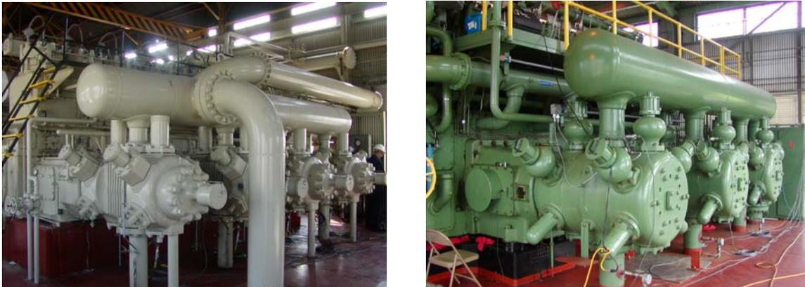
**Figure 1-1. TLA6 (2,000 HP) and GMW10 (2,500 HP) in Pipeline Service**
