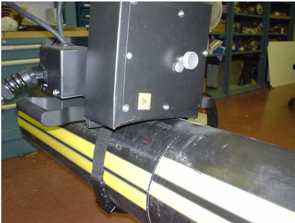
Figure 15 Inspection System on Pipe during Laser-based Inspection Phase
