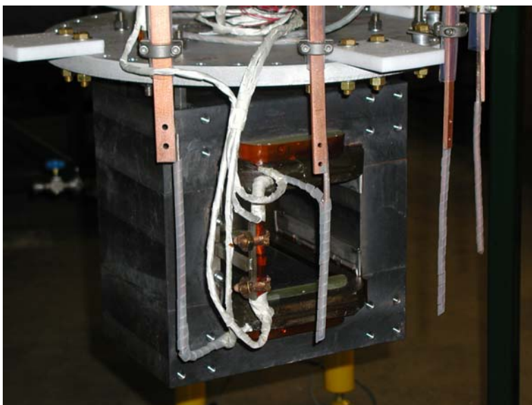
Fig. 1. Radiation tolerant dipole ready for testing.
