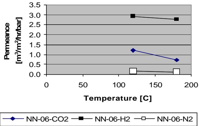
**Figure 3b Permeance vs Temperature of Carbonaceous CO<sub>2</sub>-Affinity Membranes (NN-10)**
