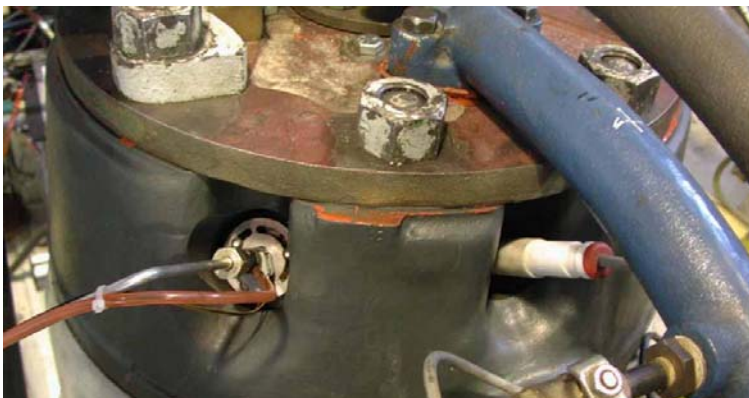
Figure 12 – GMV head with injector adapter (non-cooled)
