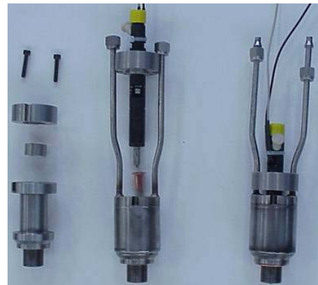
Figure 9 – Injector & adapter components
