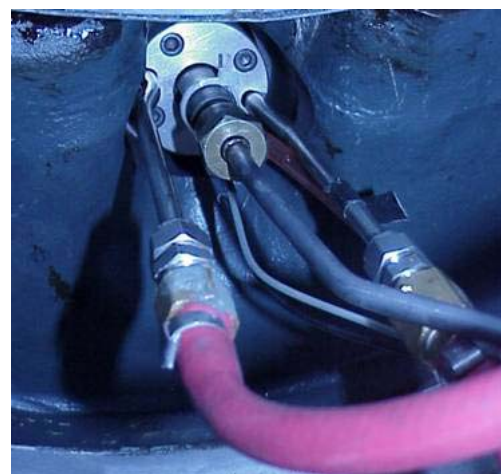
Figure 13 – injector adapter (cooled)
