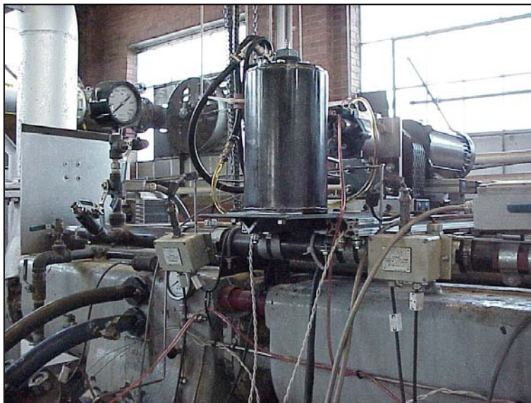
Figure 10 - Pilot fuel pump, storage, filter
