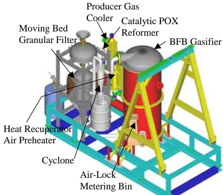
**Figure 8 Solid Model of Phase II Pilot-Scale Litter Gasification System: 12" ID reaction zone, ~120 dry lb/hr; >500,000 Btu/hr GPR. A farm-scale system would be about 3-times capacity.**
