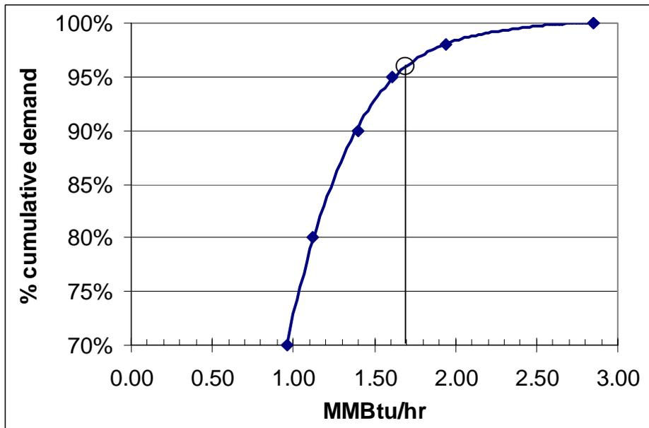
We propose that an on-farm litter gasification system be designed for a maximum litter gasification rate of 400 lb/hr. This system size would generate fuel gas at heat rates equal to 1.7 MMBtu/hr at 70% (LHV) gasification efficiency (1.6 MMBtu/hr at 65% efficiency). This scale is sufficient to meet 96% of the heat energy needs of the poultry farm. [see Fig. 8.]
