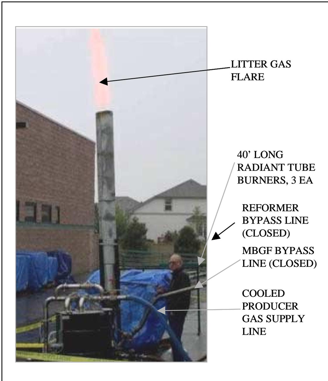
Figure 20 Flare operating on ~130 kW<sub>th</sub> producer gas from poultry litter. May 12, 2004.
