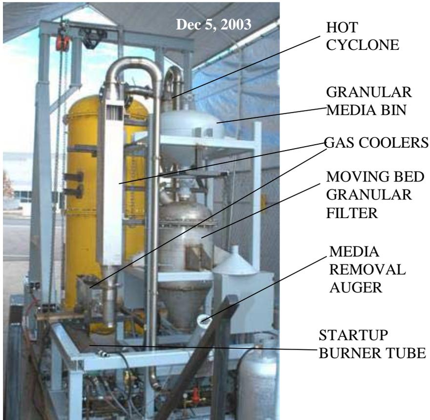
**Figure 18 Backside-View of Integrated System showing the MBGF (before insulation), cyclone, and gas coolers. Reformer and waste heat recuperator (not shown) sit in the space behind the vertical cooler.**
