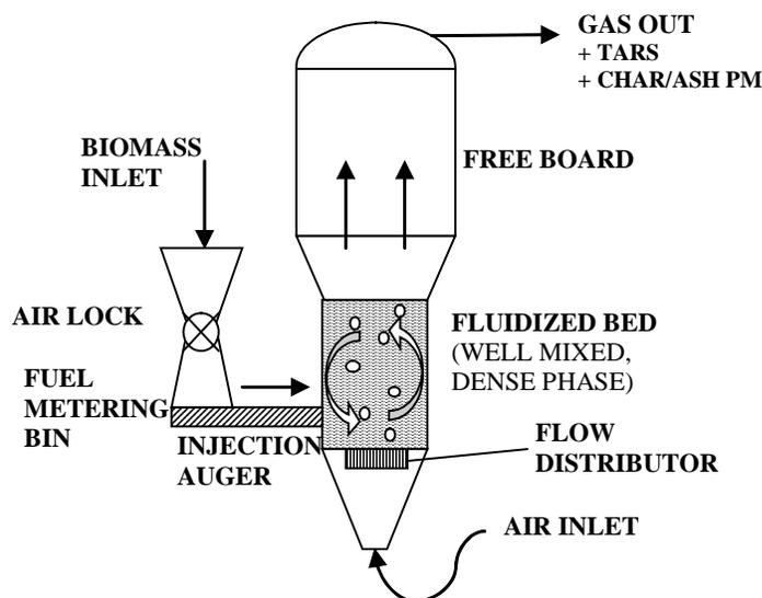
**Figure 12 Diagram of a Bubbling Fluidized Bed (BFB) Gasifier. Characteristics include a well mixed reaction zone that has less than 2% biomass mixed with hot fluidized bed media.**
