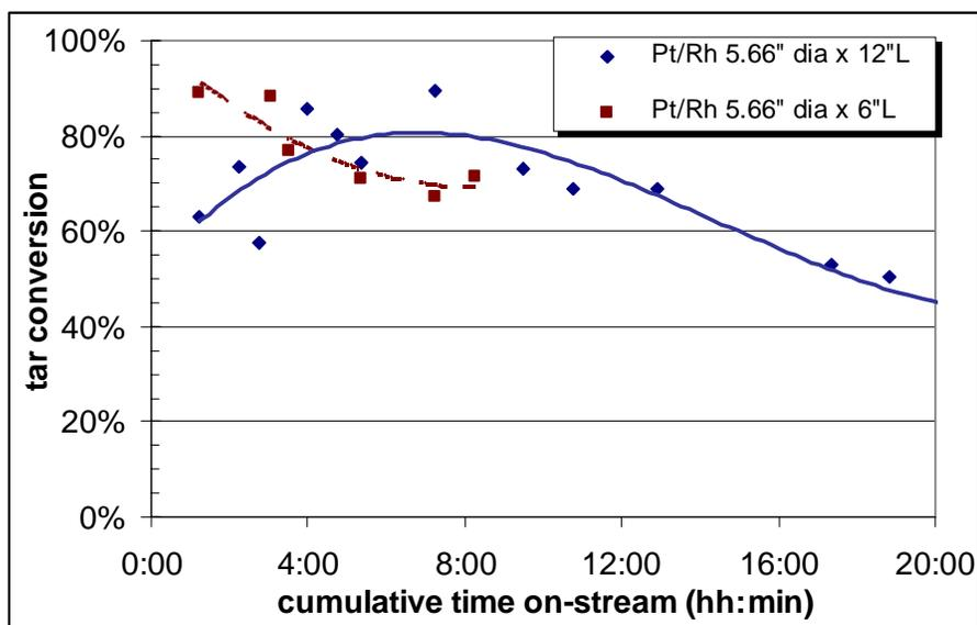
Figure 14 Plot of biomass tar conversion as a function of cumulative time on stream
