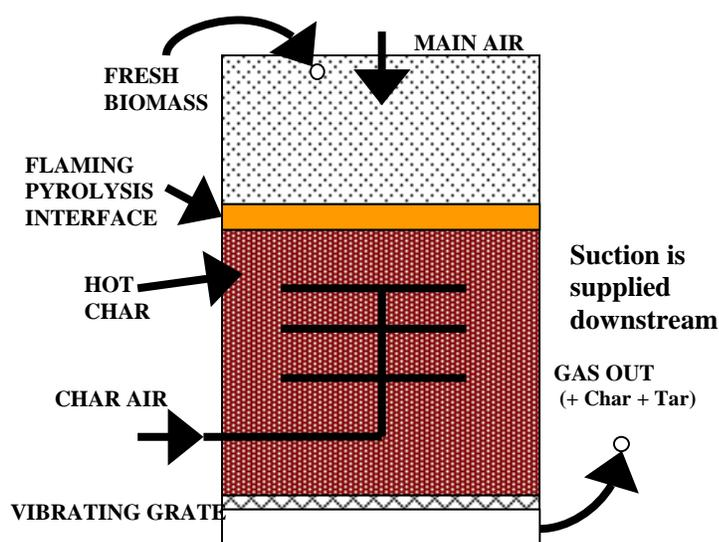
**Figure 11 Diagram of a Downdraft Gasifier with two stages of air injection (main and char-air)**
