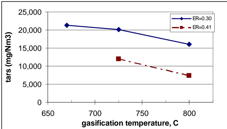
**Figure 13 ISU Lab-scale gasification tests on Poultry Litter show a logical trend. Higher temperatures and higher equivalence ratios result in lower tar yields.**
