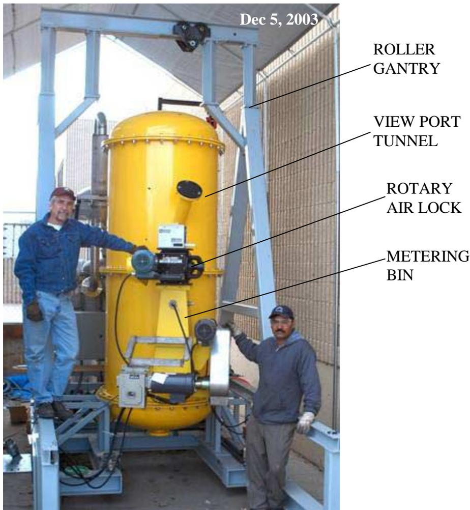
**Figure 17 Front-View of BFB Reactor showing the air lock, metering bin and view port tunnel. The view port was later modified to include and air lock hopper for adding media.**
