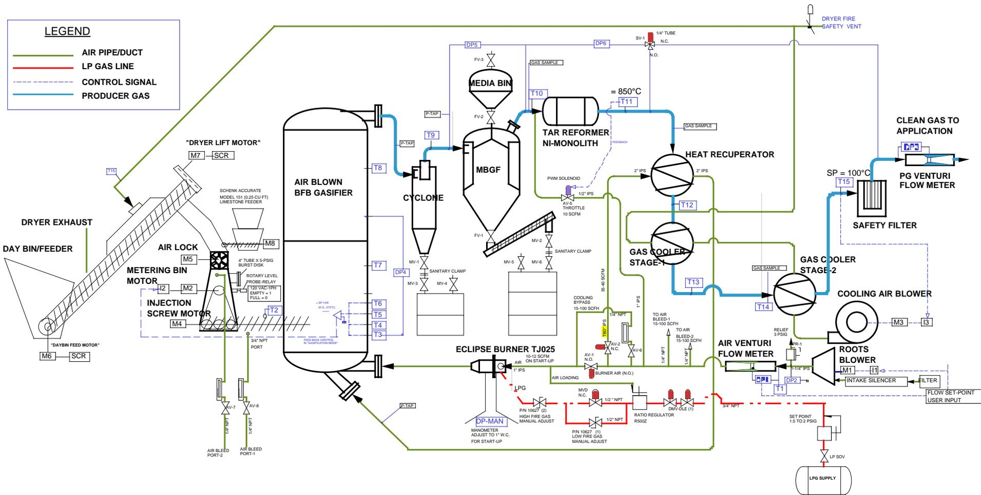
Figure 15 On-Farm Poultry Litter to Energy Gasification System, Simplified P&ID and Flow Sheet
