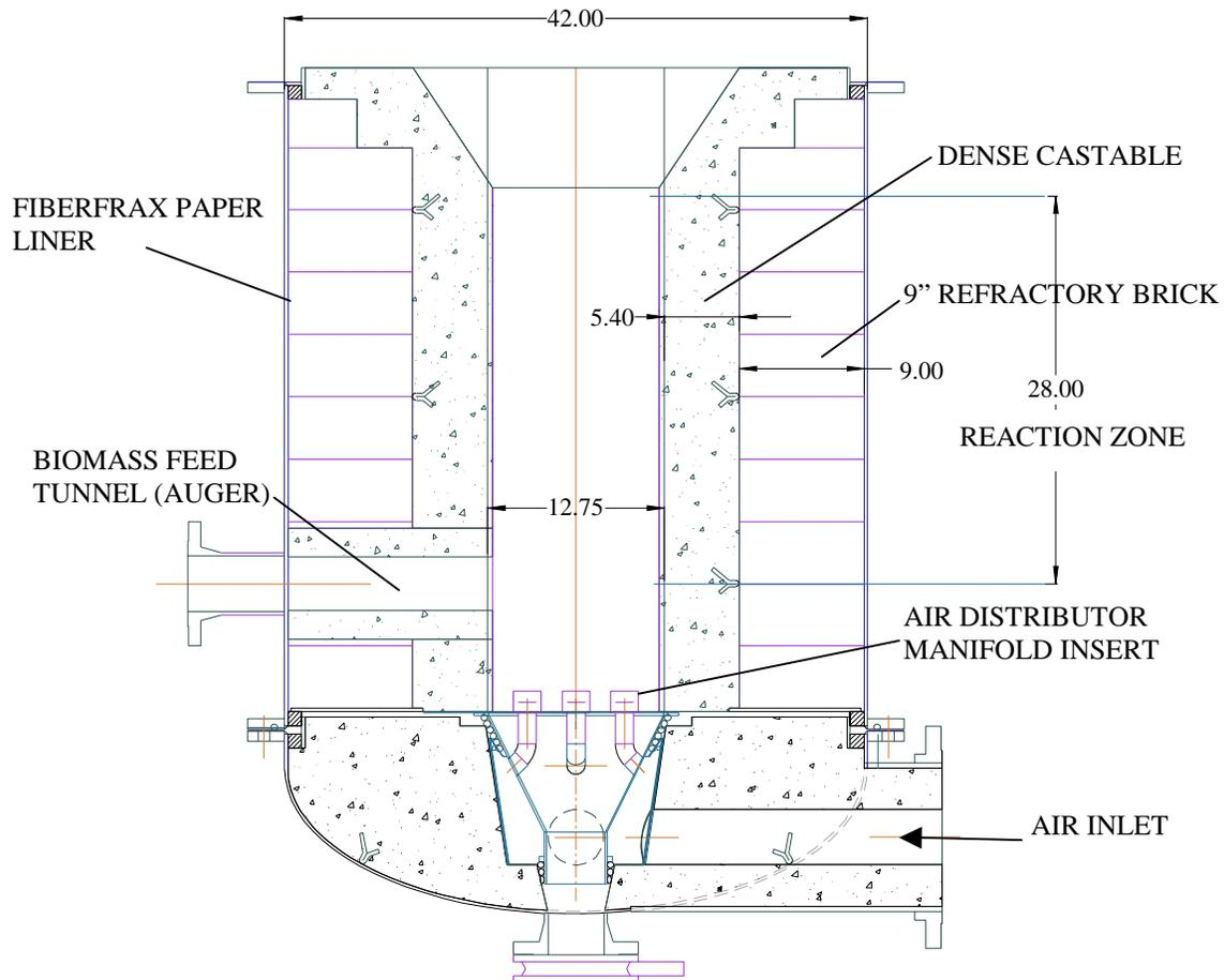
**Figure 16** Lower section view of CPC's pilot gasification vessel. The insulation design features a Fiberfrax paper liner backing a 9-inch high performance refractory brick layer, plus 5.4-inch casting erosion resistant
