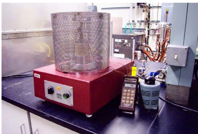
Figure 2) A view of the controlled temperature grinding system used at ASU for initial thermomechanical studies. This system is a rotary type ball mill, which has been outfitted with heating capabilities.
