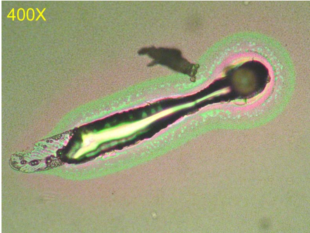
Figure 2.10 – Picture taken through a microscope of a line short, showing a typical shape for this type of short.
