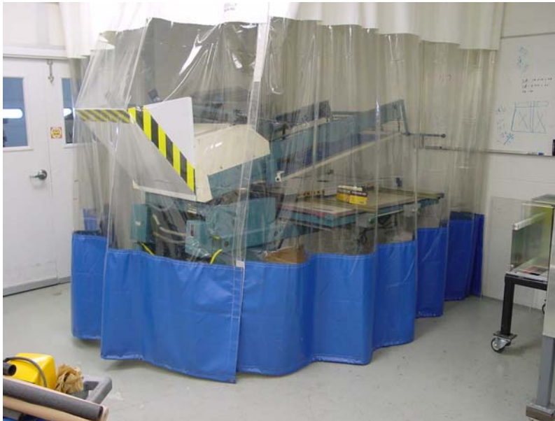
Figure 2.6 – Picture of screen printer showing the plastic shroud, and the proximity to the door discussed in the text.
