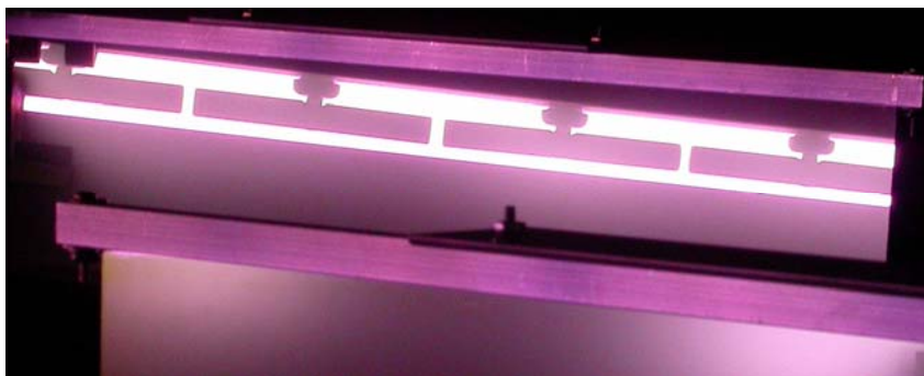
Figure 2.20 – A view of folding mirrors installed in the coater to permit real time monitoring of the plasma emission profile.
