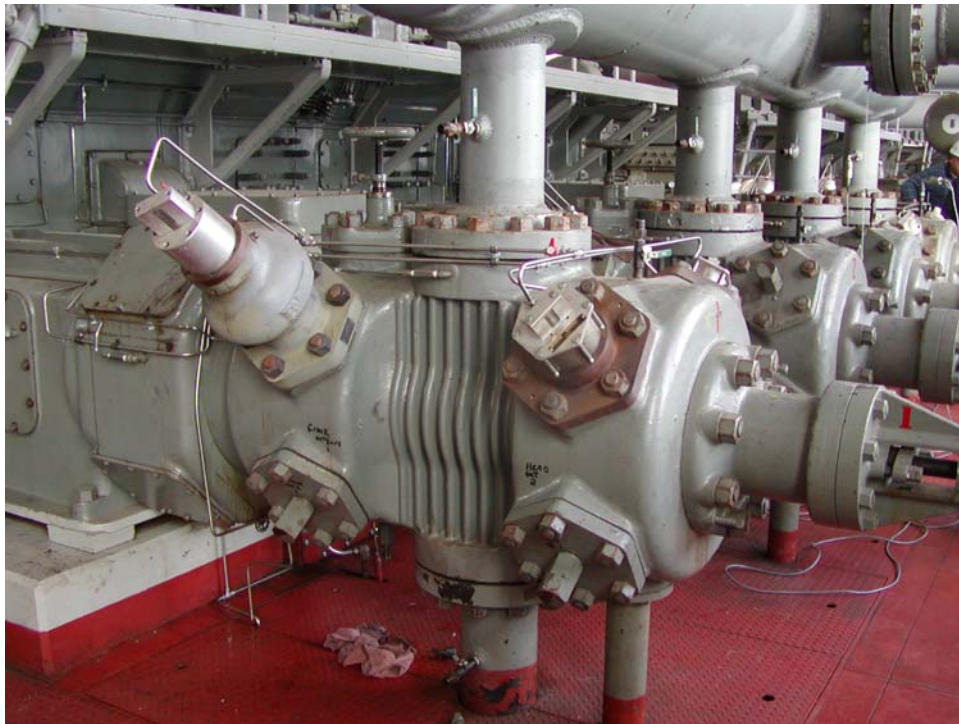
Figure 4-3. Close-up of Compressor Cylinder; Clark HBA-6 Unit (Duke Energy's Bedford Station; March 1, 2005)
