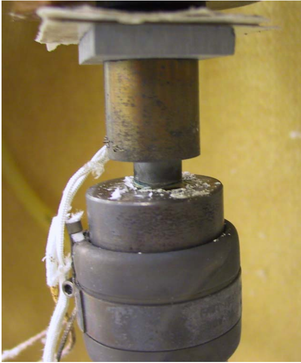
Figure 24. Glass couplant test setup prior to heating.
