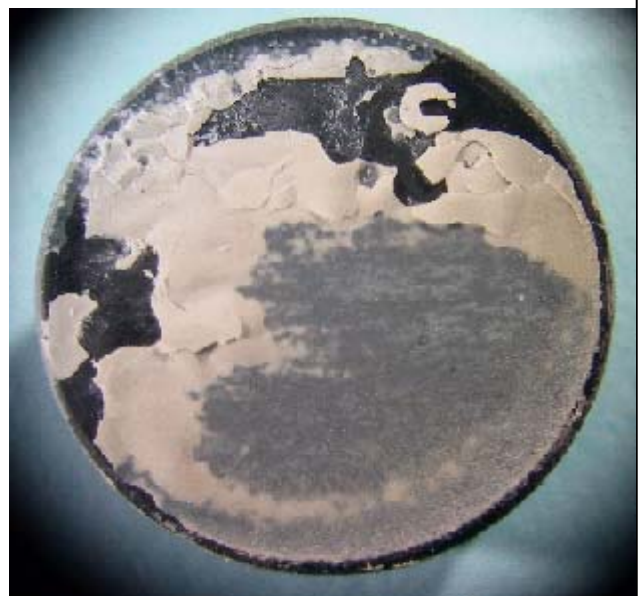
Figure 10. Polish-damaged AIN film on Performance SiC substrate.
