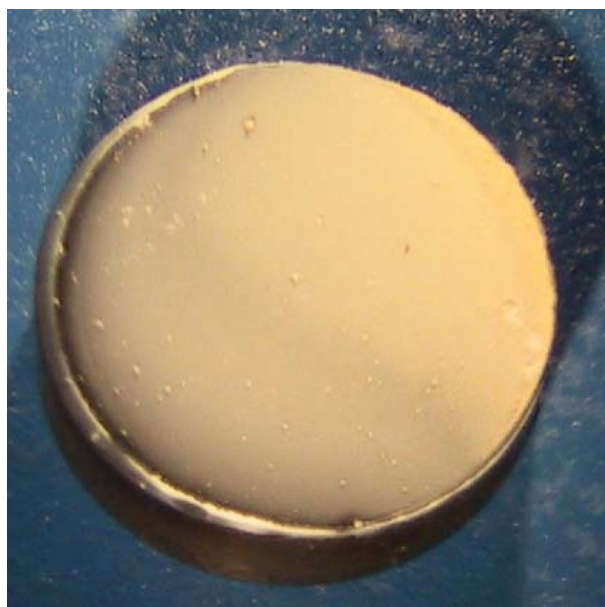
Figure 8. As-deposited AlN film on conductive bulk AlN substrate.
