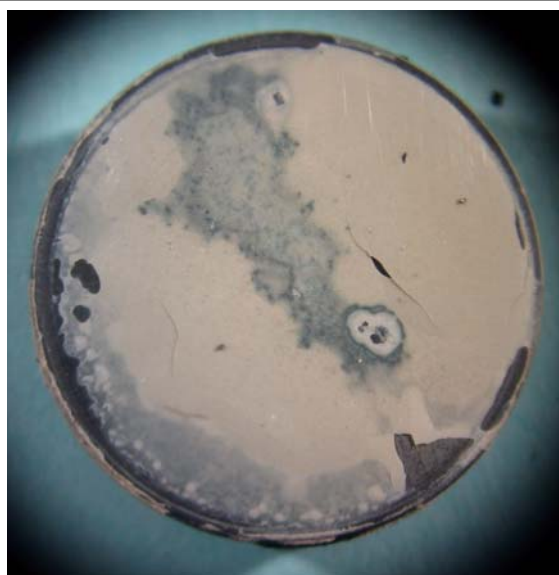
Figure 11. Delaminated AIN film on Hexoloy SG substrate after heating.
