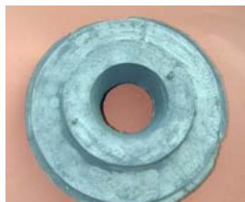
Figure 54. Disc cutter from first trial
