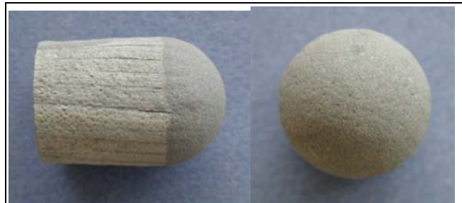
Figure 30. FM Insert after binder burnout and sintering in sand confinement
