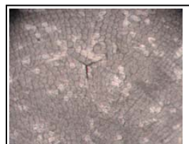
Figure 16. Exp #3, only noticeable bundle crack. Higher mag than Figure 9. Smaller microcracks probably exist.
