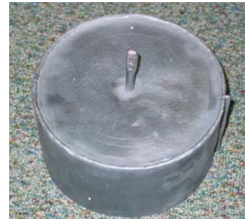
Figure 5. HIP can for disc cutters
