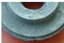
Figure 55. Crack on H13 only disc cutter
