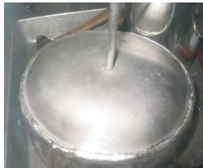
Figure 53. Blown HIP can
