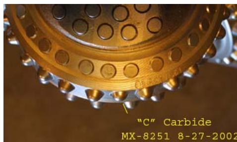
Figure 40. Drill Bit Used in Field Tests. The Superior Rock Bit test bit was 16.5 inches in diameter. The "C" carbide was the new art test insert.
