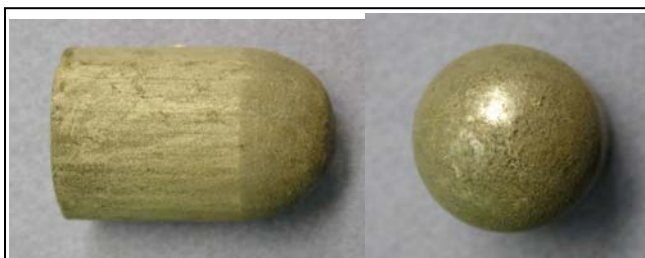
Figure 32. . FM Insert after binder burnout and sintering in container confinement with finer sand
