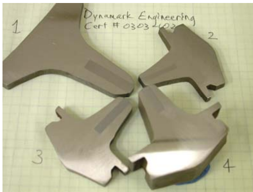
Figure 49. Disc cutter section pieces, the 17" section with the conventional WC insert is labeled 1 , a 6.5" section with a "green" FM WC insert 2 , a 6.5" section with hot pressed FM WC insert 3 , and a 6.5" section with sintered conventional WC insert 4
