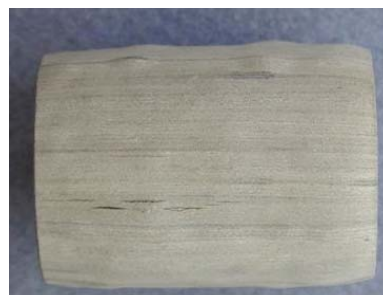
Figure 14. Cracking, delaminations, and bloating resulting from binder burnout and sintering.
