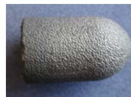
Figure 33. FM insert after container-less HIPping
