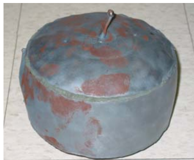
Figure 56. Blown HIP can with oxidation scaling
