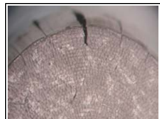
Figure 15. Sample from Exp #1. Obvious cracks, quite large and distinct. Also see cracks along bundle boundaries on top and bottom surfaces.
