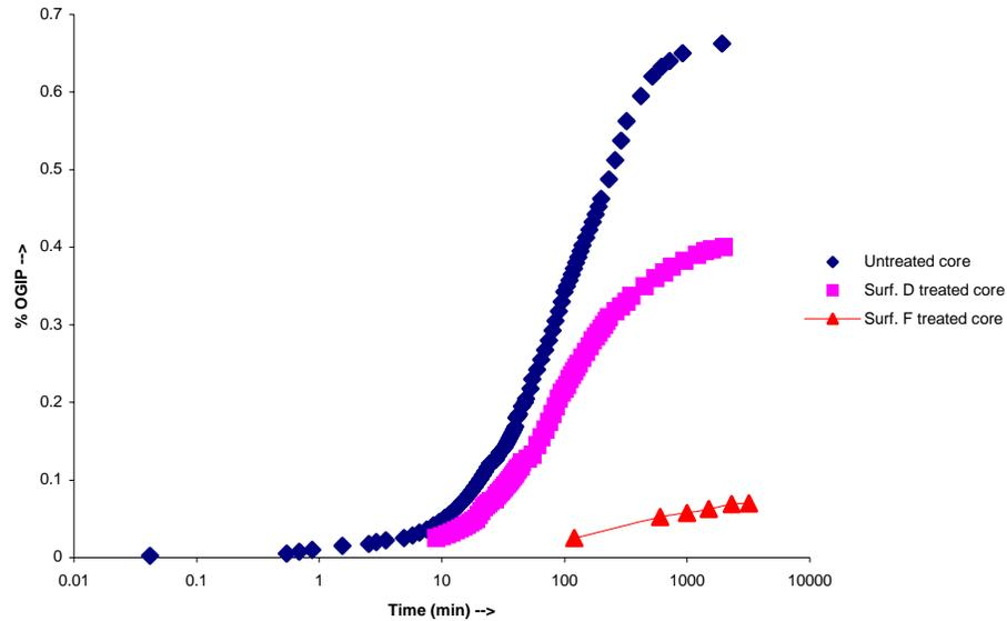
**Figure 3: Spontaneous imbibition in carbonate cores at room temperature for case of untreated core, core treated with surfactant D and core treated with surfactant F,  $S_{wi} = 0\%$ , and  $k = 120\text{ md}$ .**
