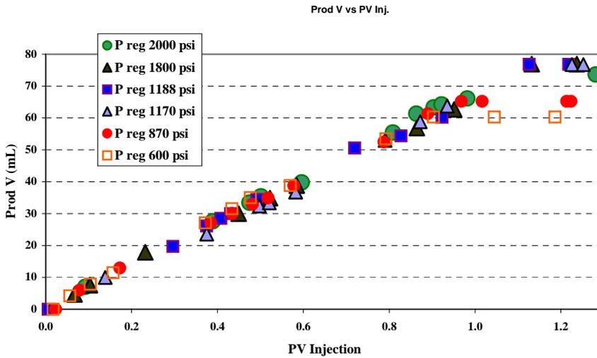
**Figure 5: Oil Production vs. PV Injection**
