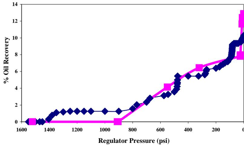
**Figure 10: Percentage Oil Recovery vs. Regulator Pressure**
