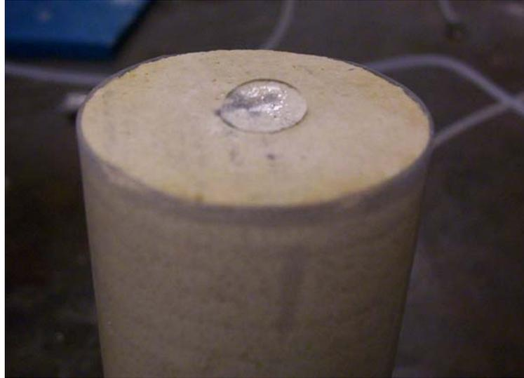
***Figure 2: Photograph of the core after treatment with surfactant F, indicating change in wettability of the surface. The drop of brine does not imbibe spontaneously into the carbonate rock.***
