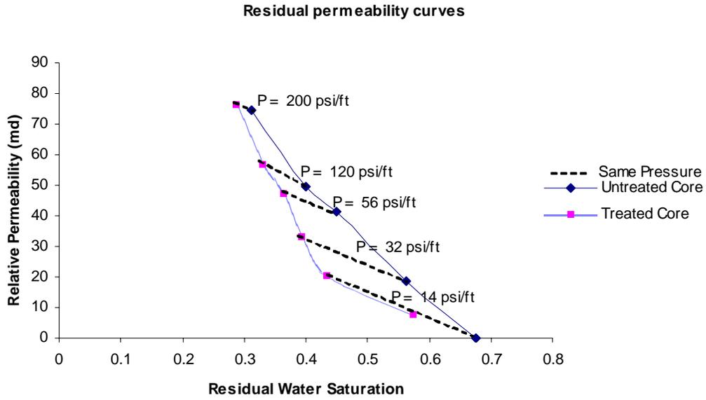
**Figure 4: Residual Permeability of Gas for Treated and Untreated Cores at Different Pressure Drops across the Core.**
