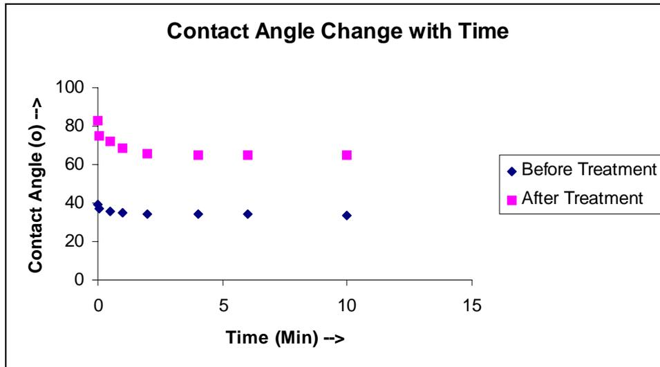
*Figure 1: Contact Angle Change with time, at large times we get equilibrium contact angle.*
