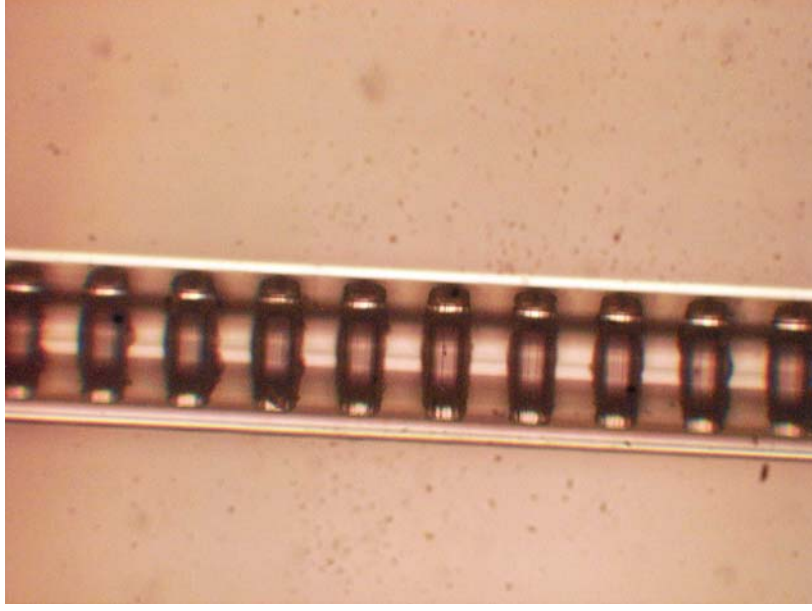
Fig. 2 Fabricate in-fiber long period grating in single crystal sapphire fiber by precise dicing.
