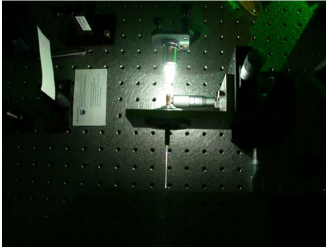
Fig. 6 Supercontinuum white light source generation for fiber sensor systems.
