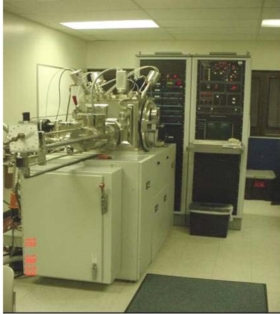
Figure 4 A picture of the DC magnetron sputtering deposition system.
