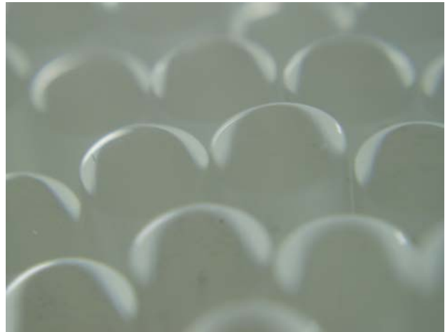
Figure 2.6. FOB polished using method two. Note the lack of debris around the edge of individual fibers.
