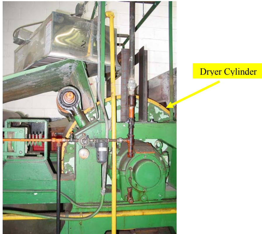
Figure 2: Close-up of Dryer Cylinder
