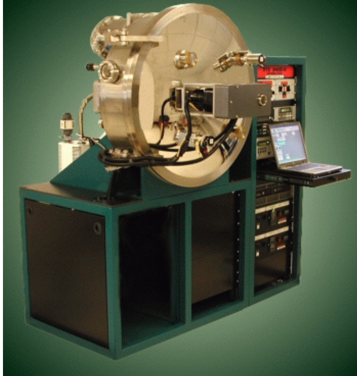
Figure 15. Hi-Z new sputtering 34" diameter chamber processes up to (6) 8" wafers, (9) 6" wafers or hundreds of small substrates with up to 4 different materials. The system shown is fitted with 400/C backside quartz lamp heating, mag-lev turbo and a dry pump.
