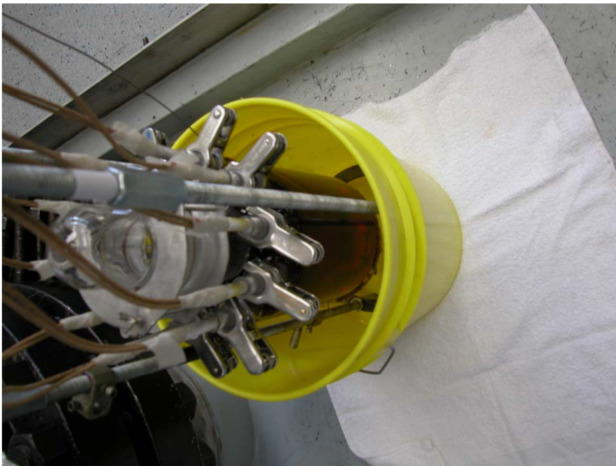
Figure 6. Glass column reboiler charged with HI solution ready for installation into pressure vessel
