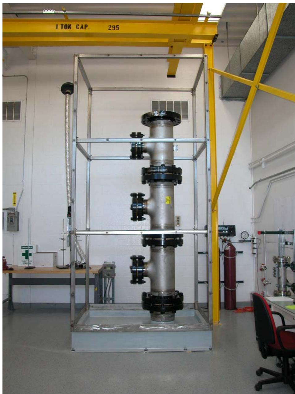
Figure 2. Pressure Vessel for Containment of Reactive Distillation Experiment.
