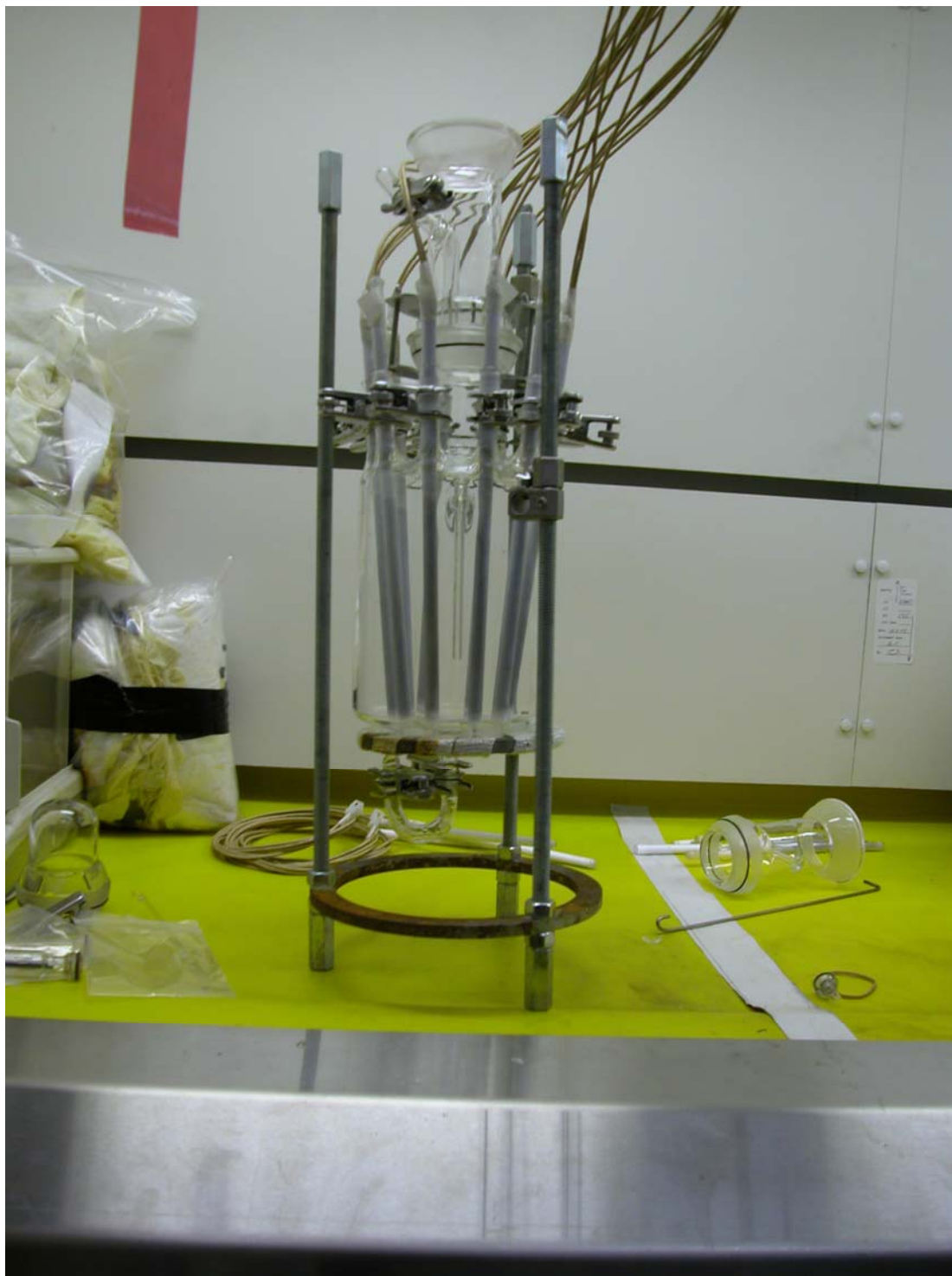
Figure 4. Glass column reboiler with quartz immersion heaters installed.
