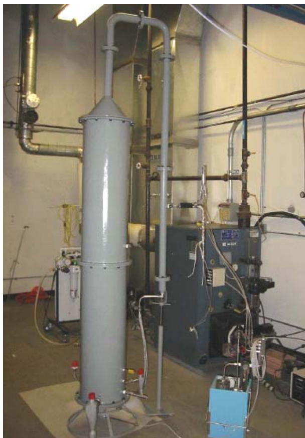
Figure 2-7. CANMET Dilution Sampler Version 3 (Lee et al., 2003).
