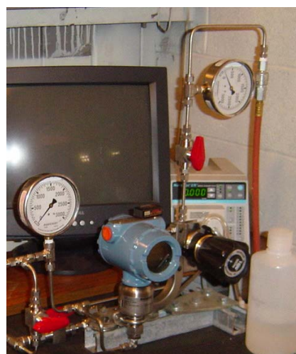
Fig. 3.4 Air and liquid injection systems
