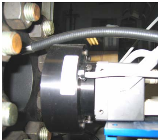
Fig. 7.7 CCD camera with fiber light and ring light installed
