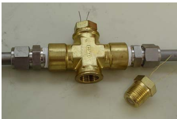
Fig. 7.8 Prototype device for measuring the average bubble size of foam
