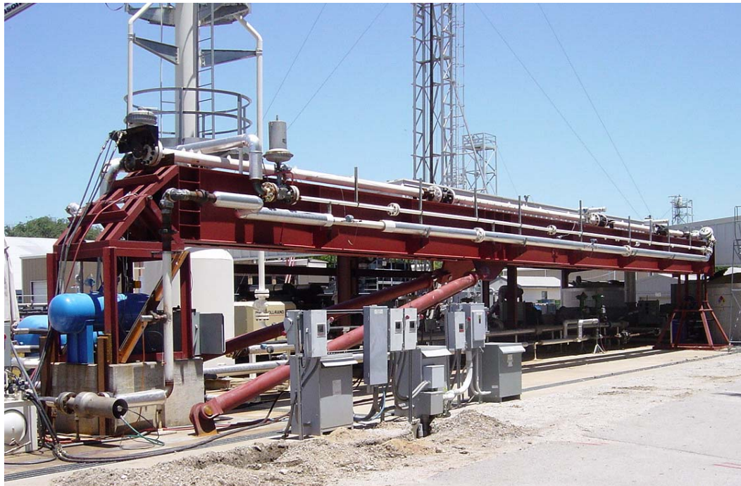
Fig. 2.1 Mast together with the hydraulic cylinders
