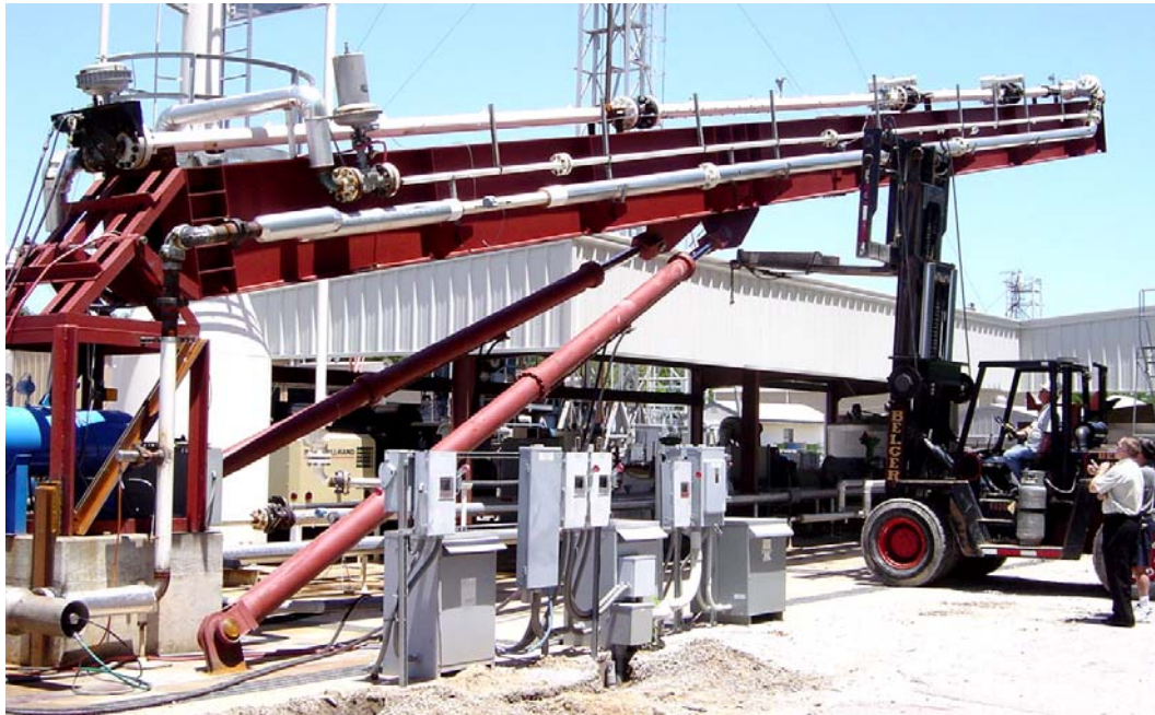
Fig. 2.2 Mast when raised approximately 10 degrees
