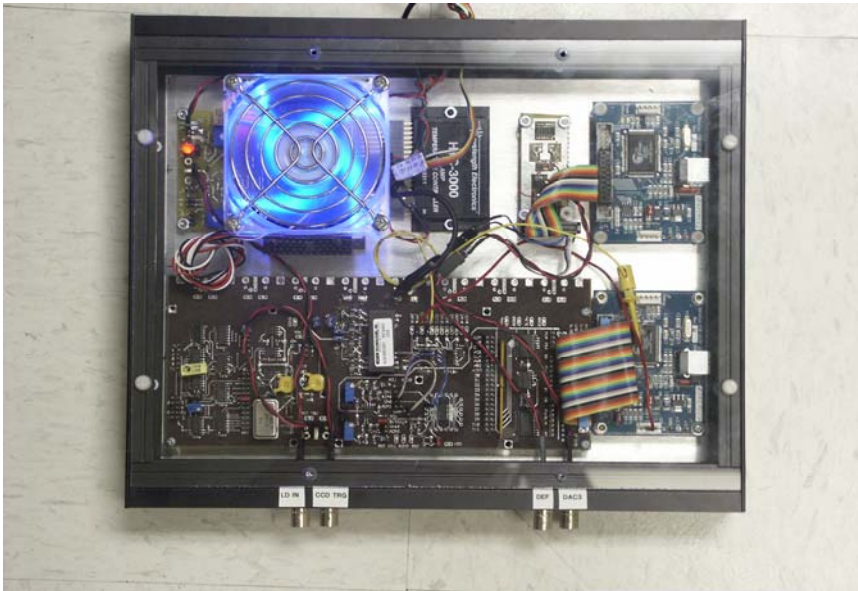
Figure 2. For field use, integrated CCD controller and lower power diode laser and DPSSL laser controller with programmable pre-pumping capability.
