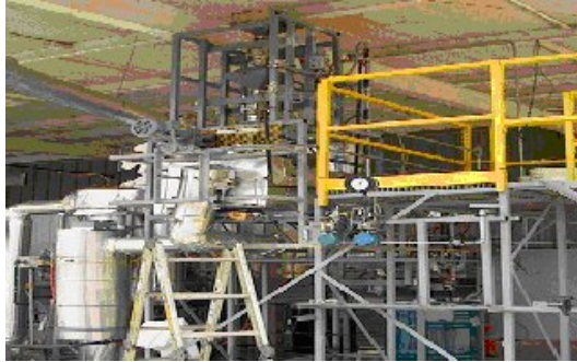
Figure 5 Pyrolizer with Biomass feedstock system
