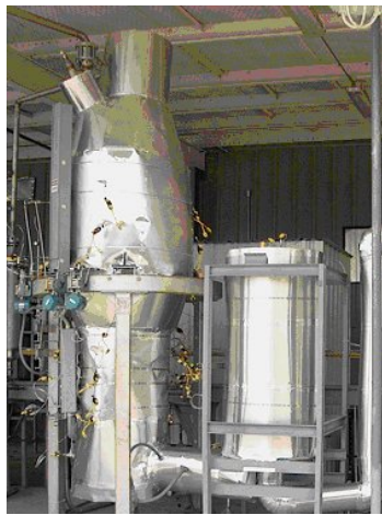
Figure 6 Reformer and Vapor Heater
