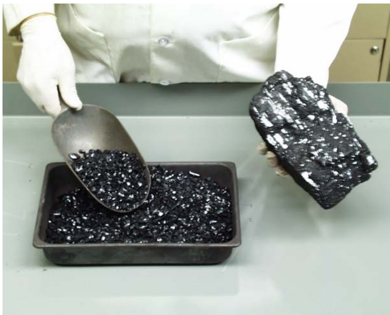
Figure 2. Left, WVU coal-extract binder after dissolution and solvent extraction of Bakerstown coal; Right, Bakerstown coal prior to extraction.
