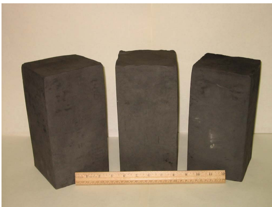
Figure 5. Photograph of representative graphite billets.
