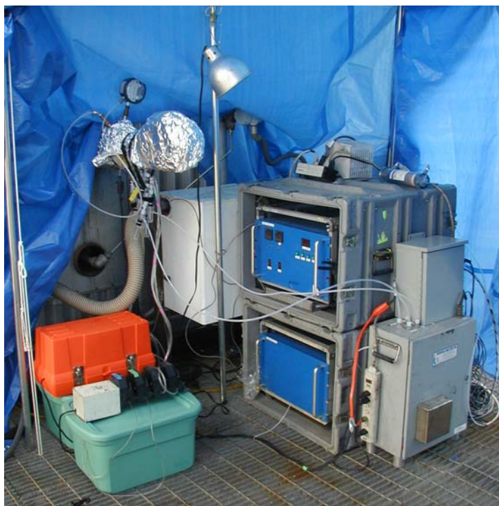
Figure A-2. Photograph of Apogee mercury S-CEM installed at a field site.
