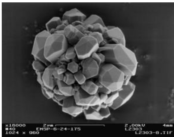
Aggregate of hexagonal cancrinite crystals formed after 24 hr of reaction at 175 °C under low Si (0.01M), high Al (0.5M), and high OH (4.5M) conditions.
