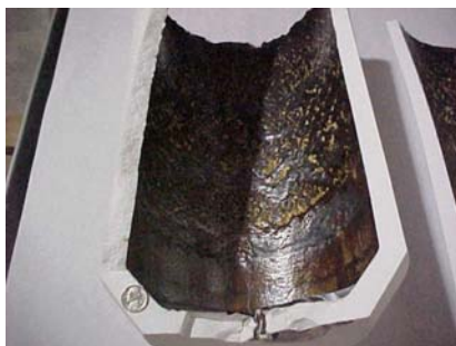
Figure 10. Cross sectional view of a dense high silica crucible after 14 days at 1250°C with the iron phosphate melt containing 27 wt% LAW (IP27LAW).
