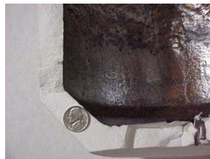
Figure 10. Cross sectional view of a dense high silica crucible after 14 days at 1250°C with the iron phosphate melt containing 27 wt% LAW (IP27LAW).
