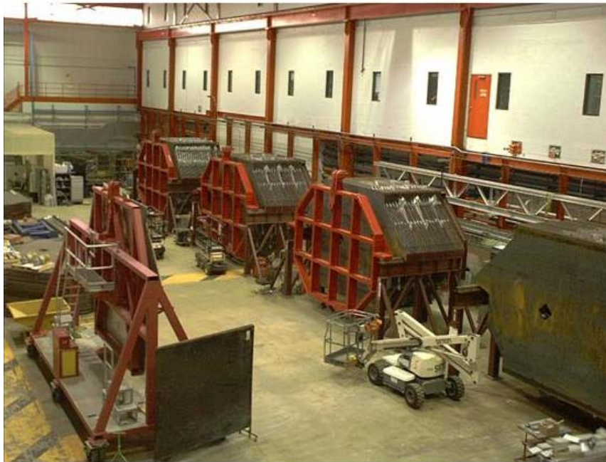
Figure 2. The MINOS near-detector planes in the New Muon Lab at Fermilab. The four storage racks along the wall in the background contain the assembled steel and scintillator planes. The planes in the storage rack at the far left are being used for the nine-plane commissioning test. The plane-installation transport fixture, which will carry planes from the underground shaft station to the near-detector hall, can be seen in the lower left corner of the photograph.
