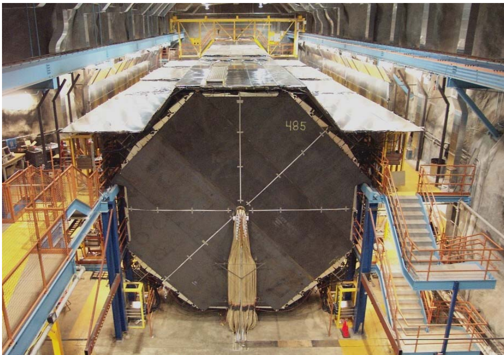
Figure 1. The completed MINOS far detector. The photograph shows the MINOS far detector at Soudan in July 2003, following the completion of installation, including the magnet coil and the cosmic-ray veto shield. The coil wires and cooling water tubes can be seen emerging from the central hole in the last steel detector plane. The large aluminum-covered panels above the detector are the scintillator modules that make up the completed top section of the veto shield. The nearly completed side sections of the shield, constructed of vertical and 45 degree panels, can be seen along the sides of the detector.
