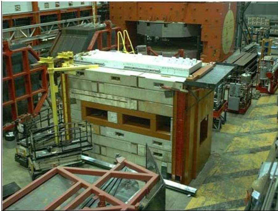
Figure 3. NuMI hot work cell preassembly at Fermilab. The photograph shows the concrete and steel hot work cell after preassembly in the New Muon Lab at Fermilab. The hot work cell will be used to work on NuMI beamline production-target and magnetic-horn assemblies that develop faults after becoming radioactive. The four apertures in the walls of the structure (three in the concrete-block sidewall and one in the steel endwall) will be filled with lead glass to provide a clear view of radioactive components. Usually a faulty target or horn will not be repairable but must be replaced with a spare unit using the remotely controlled devices in the hot work cell.
