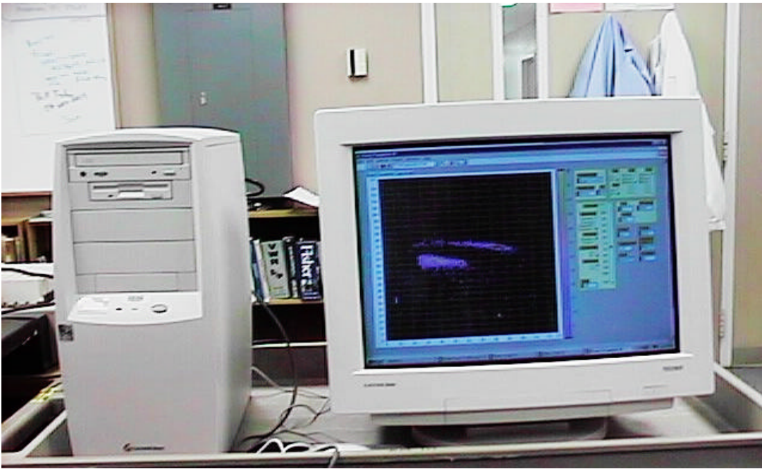
Figure 10. Photo of Digital Data Acquisition System. The digital oscilloscope resides in the computer.
