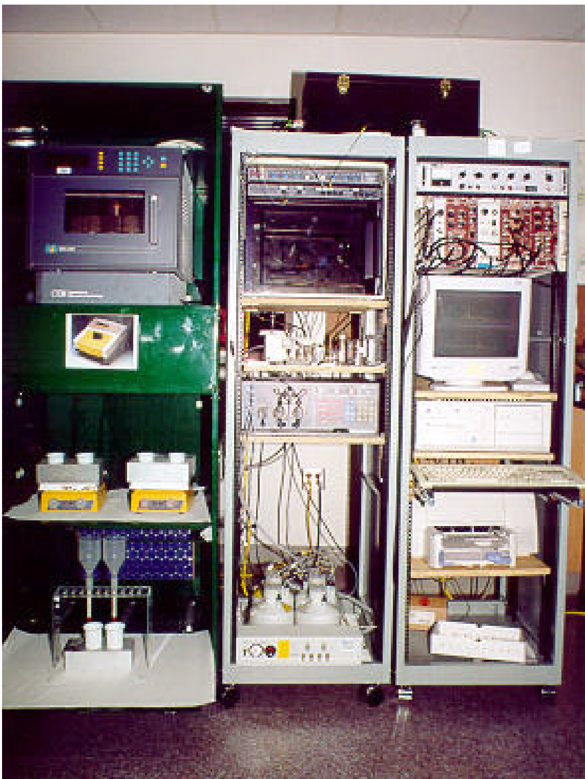
Figure 9. Photograph of the laboratory prototype. The left cabinet is for sample processing, the middle cabinet houses the ion chromatography system and the right cabinet contains the analog pulse shape discrimination system. The flow-cell is housed in the black box that is atop the middle and right cabinets.
