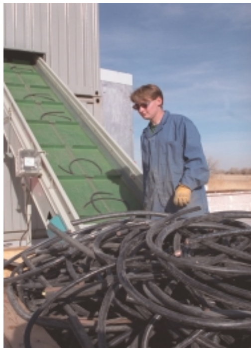
Figure 3. Placing cables on the conveyor to the shredder.
