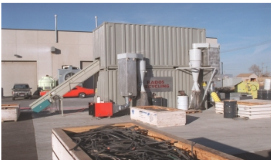
Figure 1. RADOS Copper Cable Recycling Technology provided by NUKEM and installed for the demonstration tests at the INEEL.
