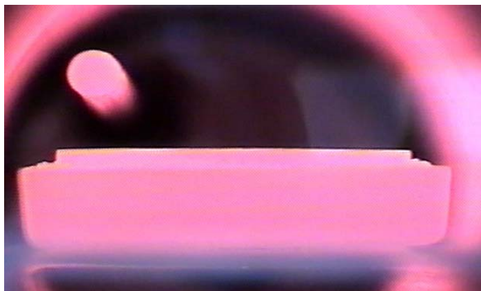
Figure 8: \text{Na}_2\text{CO}_3 drop on mullite specimen after melting
