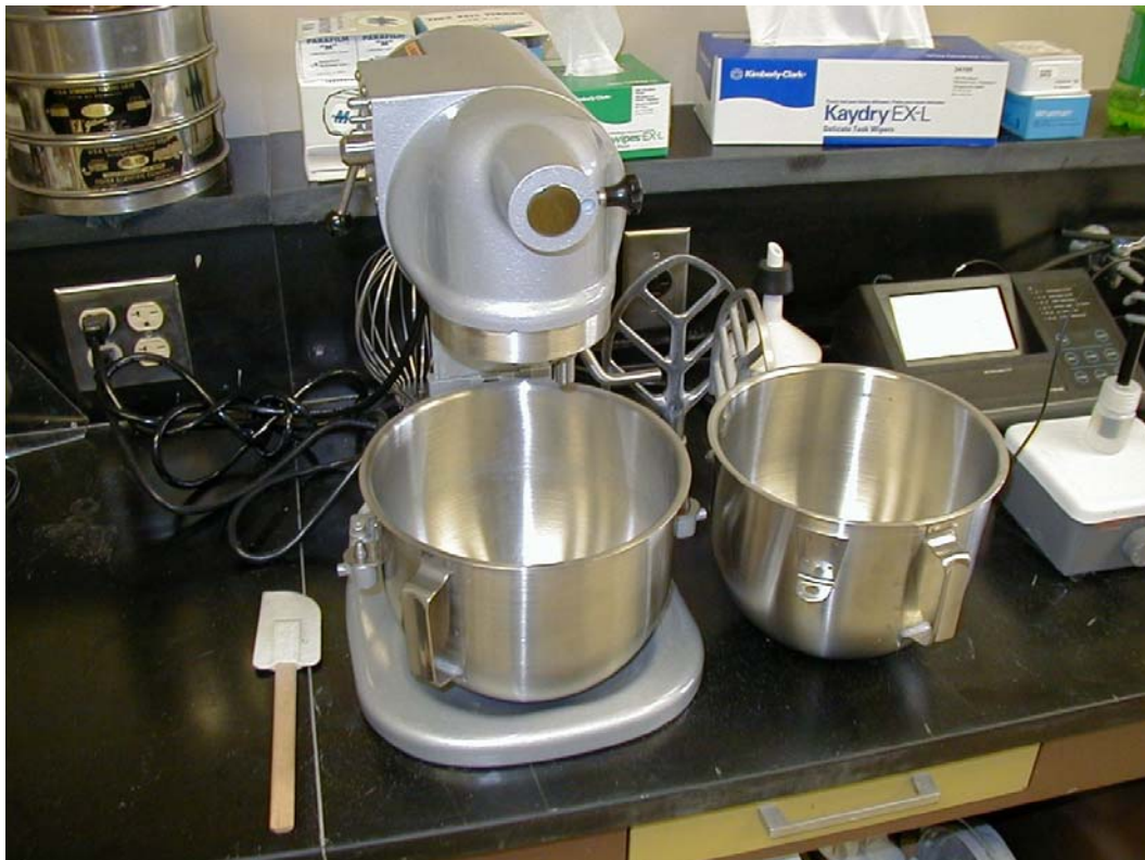
Figure 1. Laboratory mixer used to prepare mortar.
