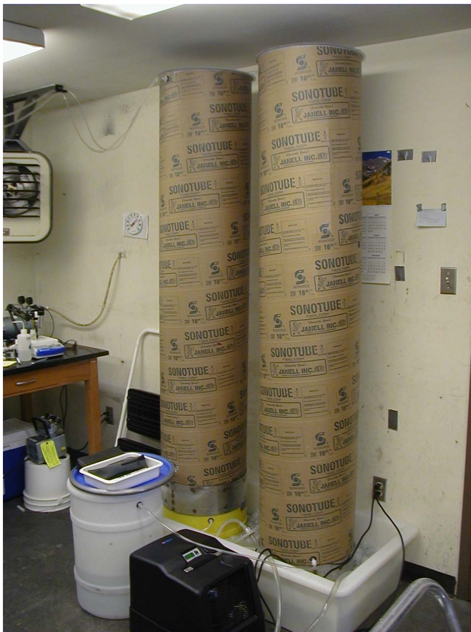
Figure 1. Sonotube apparatus used to measure long-term ammonia loss from concrete.
