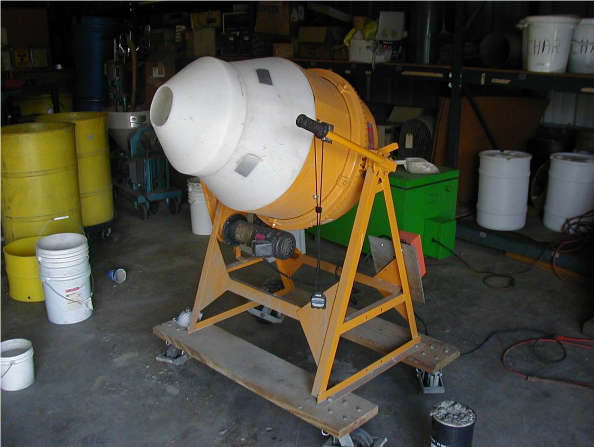
Figure 2. 3.5 cu. ft. mixer modified to simulate a commercial Ready Mix truck mixing drum.
