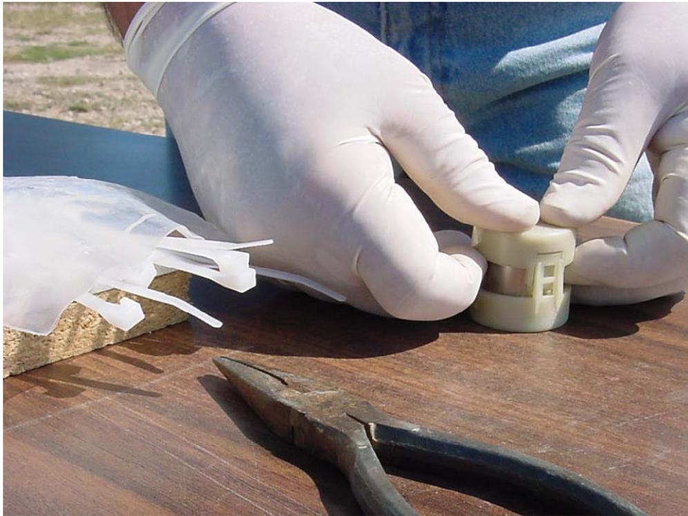
**Figure 3. Accu Core Sampler Being Sealed**
