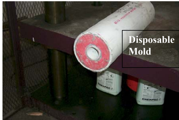
Figure 10: Support Cast into Disposable Mold
