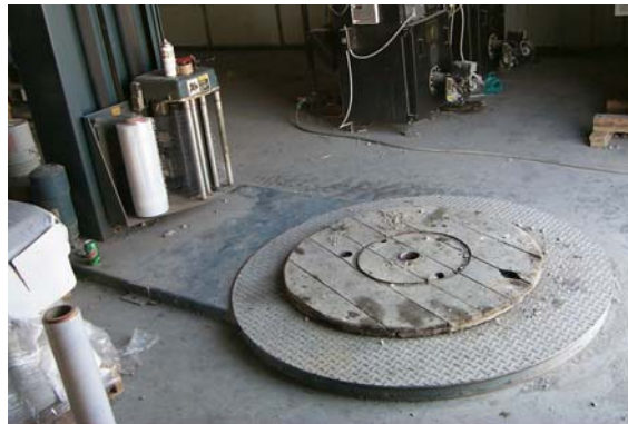
Figure 14: Packaging Wrapper and Turntable for Stretch Wrapping
