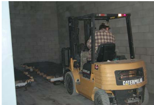
Figure 12: Fork-Lift Truck Operation Putting Filled Molds in Curing Chamber
