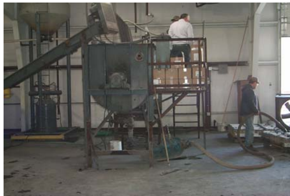
Figure 7: Wet Mixer, Fly-Lite, Inc.
