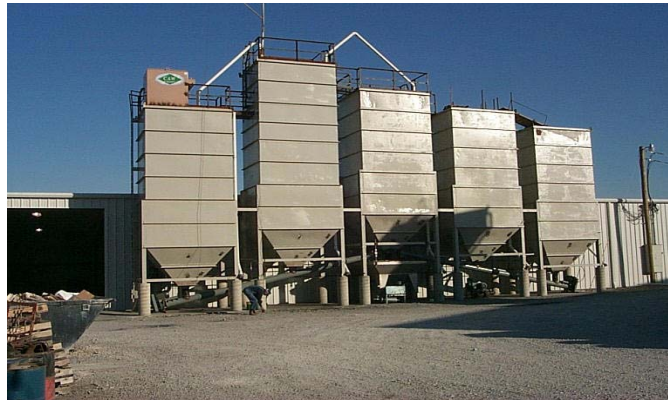
Figure 3: Silos for Storage of Fly Ash and Binders
