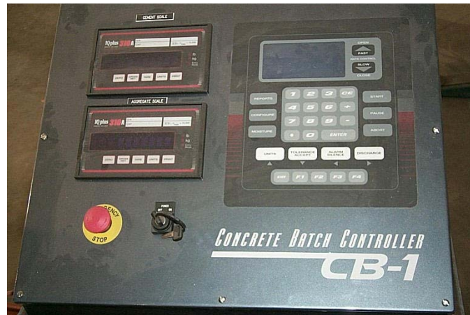
Figure 15: Programmable Control Systems for Pilot Scale Facility
