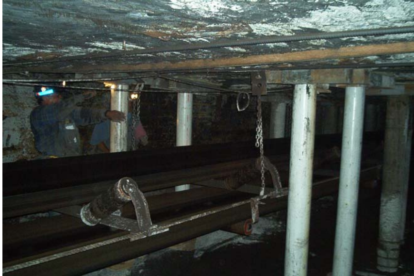
Figure 43: Field Demonstration of Composite Posts in a Central Illinois Coal Mine
