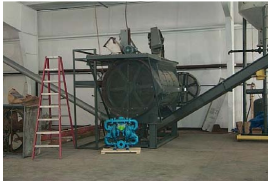
Figure 5: Dry Mixer with Screw Conveyors at Fly-Lite, Inc.
