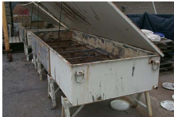
Figure 25: Large Size Hot Water Curing Tanks for Crib and Post Elements
