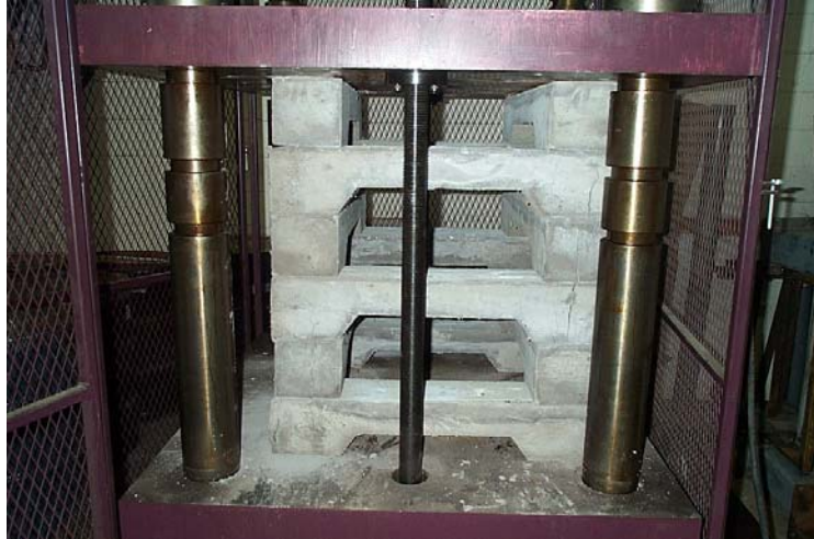
Figure 37: Prototype Second Generation Crib Element in the Test Frame
