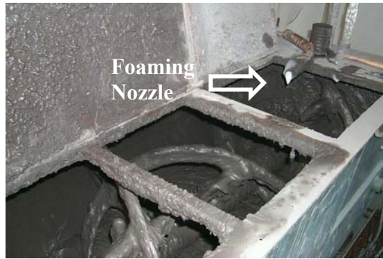
Figure 8: Wet Mixer Operation, Fly-Lite, Inc.
