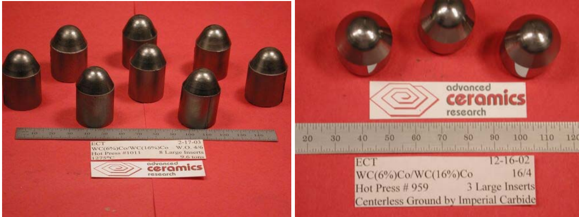
Figure 9 – Hot pressed WC-Co(6%)/WC-Co(16%) FM drill bit inserts before (left) and after (right) centerless grinding.
