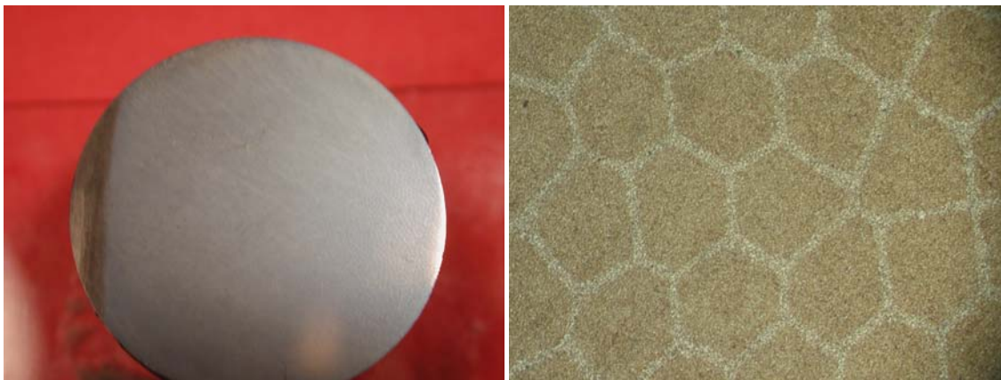
Figure 10 – Cross section of hot pressed WC-Co(6%)/WC-Co(16%) FM drill bit insert at 5X (left) and 50X (right).
