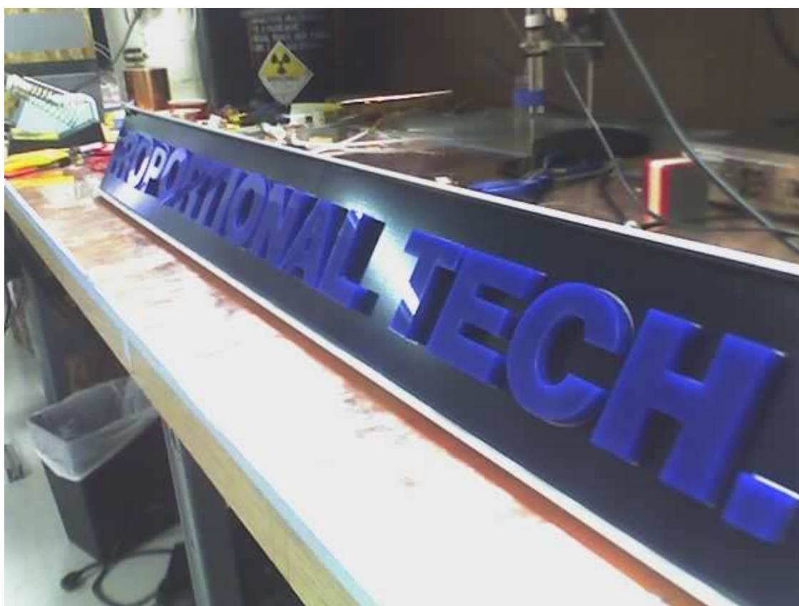
Figure 28: Acrylic letter collimator.
