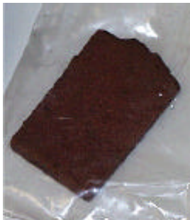
Figure 4. Photograph of ^{235}\text{U} sample for imaging test. Its dimensions are \sim 2 \times 3 cm.
