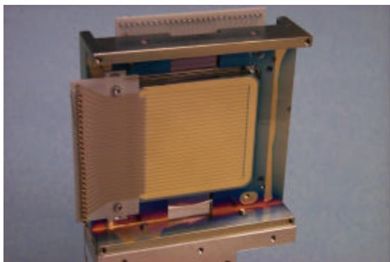
Figure 1. Full sized Ge detector with amorphous contacts. Each side has 25 strips with 2 mm pitch.
