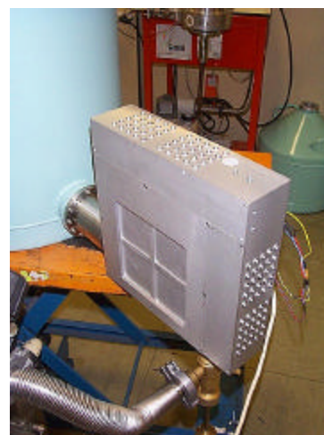
Figure 2. Array of 4 Ge detectors in cryostat. The 2 \times 2 array has 2 mm position resolution.
