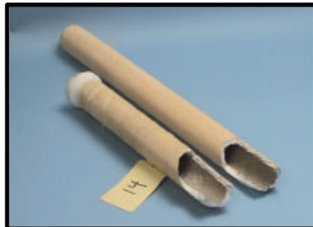
Figure 51 — Failure of the vacuum infiltrated chopped fibrous candle filters.
