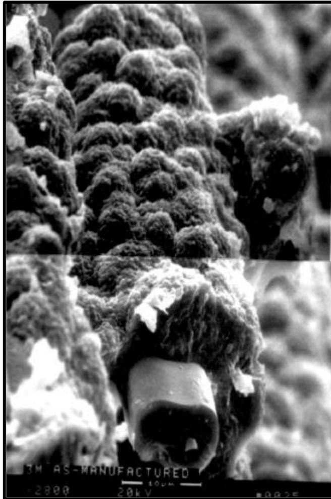
Figure 40 — CVI-SiC layer deposited along the outer surface of the 3M Nextel™ 312 structural support triaxial braid.
