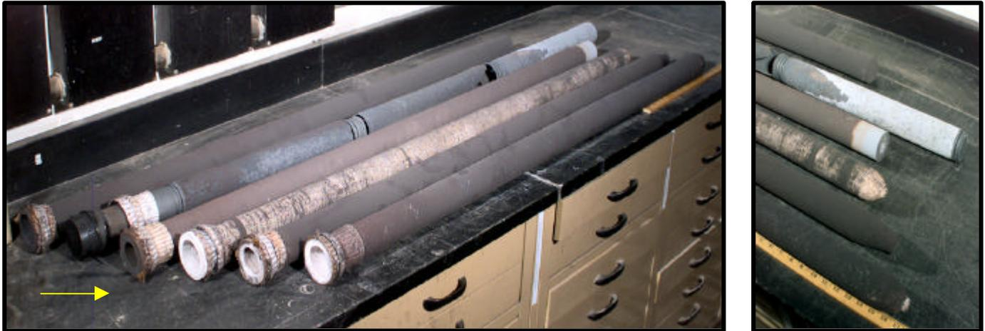
Figure 67 — Candle filters at the conclusion of Test Segment No. 2 — 486 hours of exposure at 840°C (1550°F) in the simulated PFBC process gas environment containing gas phase sulfur and alkali. Elements from left to right include: Filtros recrystallized SiC; Pall iron aluminide; Schumacher clay bonded SiC FT20; Techniweave CFCC; DuPont PRD-66; and McDermott CFCC.
