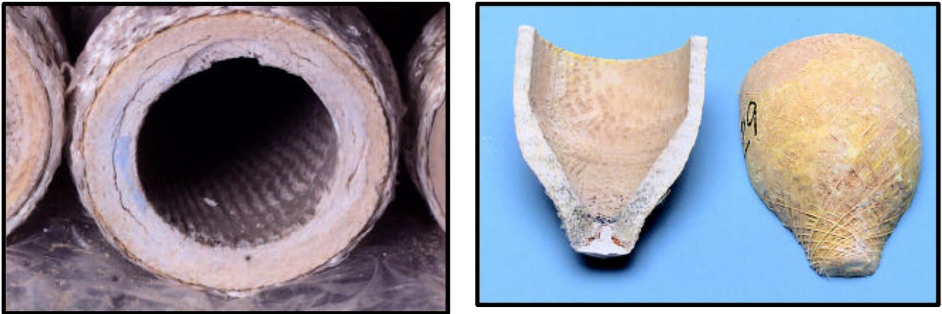
Figure 57 — Critical inserts within the McDermott CFCC filter element.
