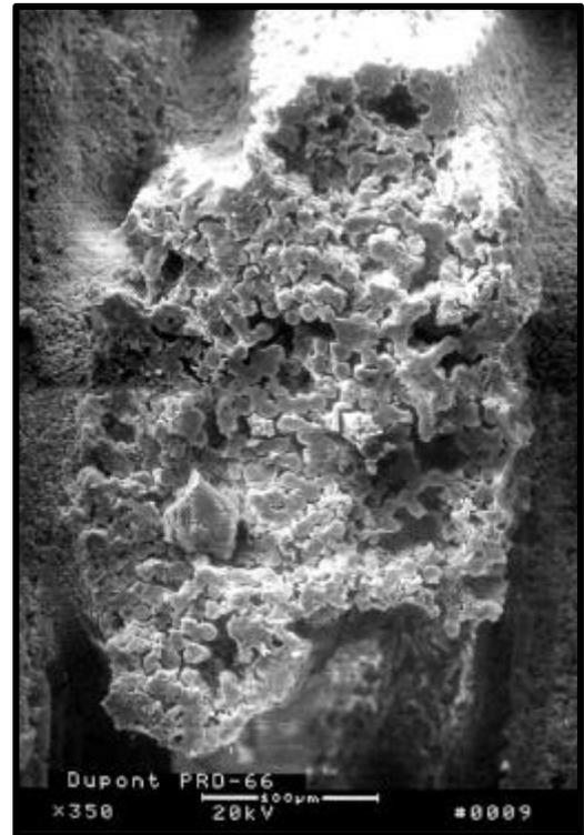
Figure 72 — Microstructure of the DuPont PRD-66 filter matrix after 486 hours of exposure to the gas phase alkali and sulfur-laden, 840°C (1550°F), simulated PFBC process gas environment. In comparison to an as-manufactured DuPont PRD-66 filter matrix, negligible microstructural changes were detected.
