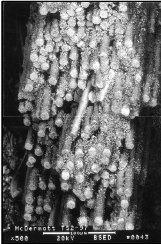
Figure 36 —Nextel™ filament bundles contained within the McDermott CFCC candle filter.
