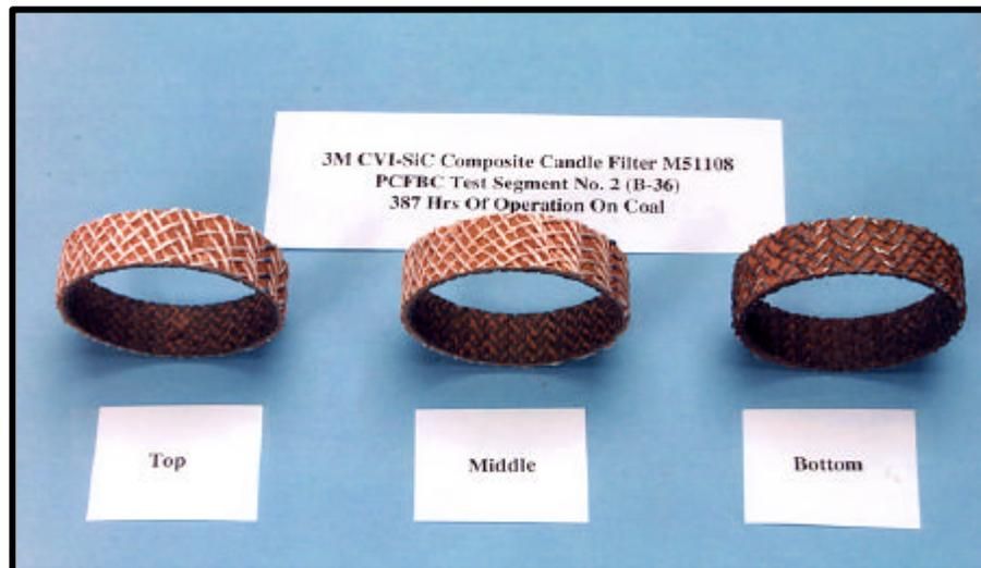
Figure 41 — Sections of the 3M CVI-SiC composite candle filter after PFBC or PCFBC operation.
