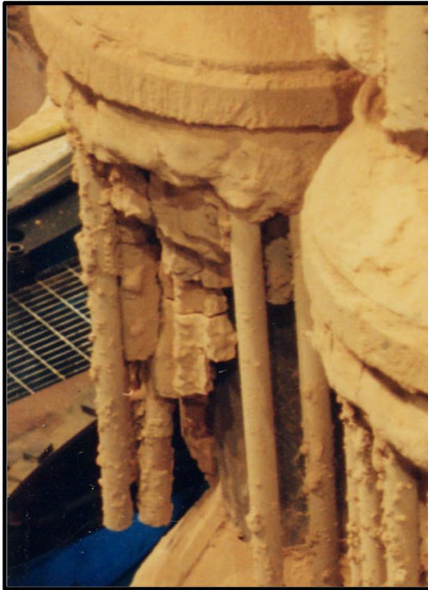
Figure 50 — Failure of the porous ceramic filter elements as the result of ash bridging within the filter array.
