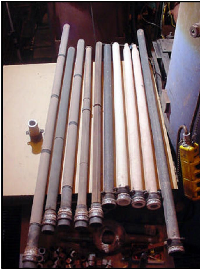
Figure 65 — Filter elements at the conclusion of steady state, accelerated pulse cycling and thermal transient testing. From left to right: 2.0 m Pall FeAl; 1.5 m U.S. Filter/Fluid Dynamics 316L; 1.5 m Pall FeAl; 1.5 m Bekaert/Mott Fecralloy; 1.5 m Microfiltrex Fecralloy metal media filter elements; 1.5 m Filtros recrystallized SiC; 1.5 m Techniweave CFCC; two 1.5 m DuPont PRD-66; and 2.0 m Filtros recrystallized SiC ceramic filter elements.
