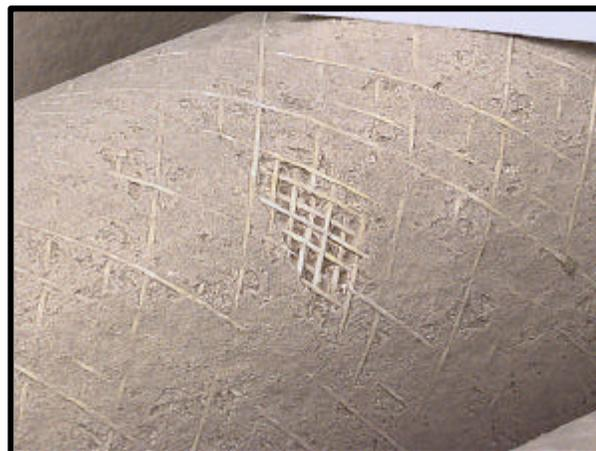
Figure 56 — Removal of fibers along the outer surface of the McDermott CFCC filter element.
