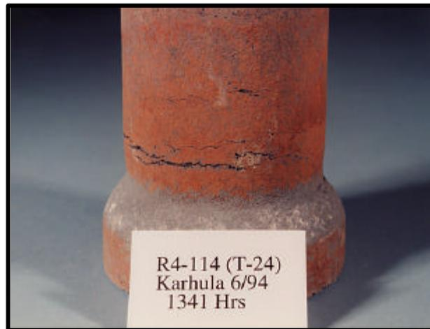
Figure 49 — Crack formations at the base of the Pall Vitropore filter flange as a result of high temperature creep during operation at AEP.
