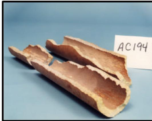
Figure 47 — Thermal fatigue of the Coors P-100A-1 alumina/mullite filter matrix.
