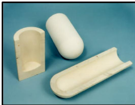
Figure 48 — Coors P-100A-1 alumina/mullite closed end cap. Radiusing of the filter wall in the end cap region eliminated stress risers within the matrix, mitigating failure of the filter body.
