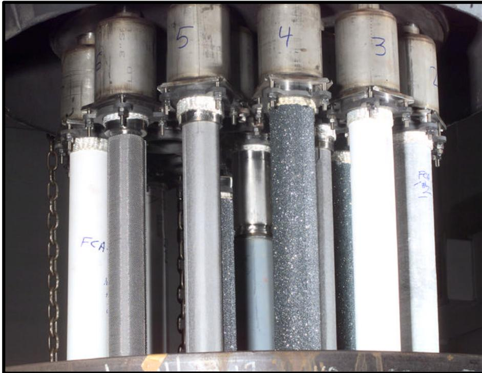
Figure 63 — Ceramic and metal candle filter array.
