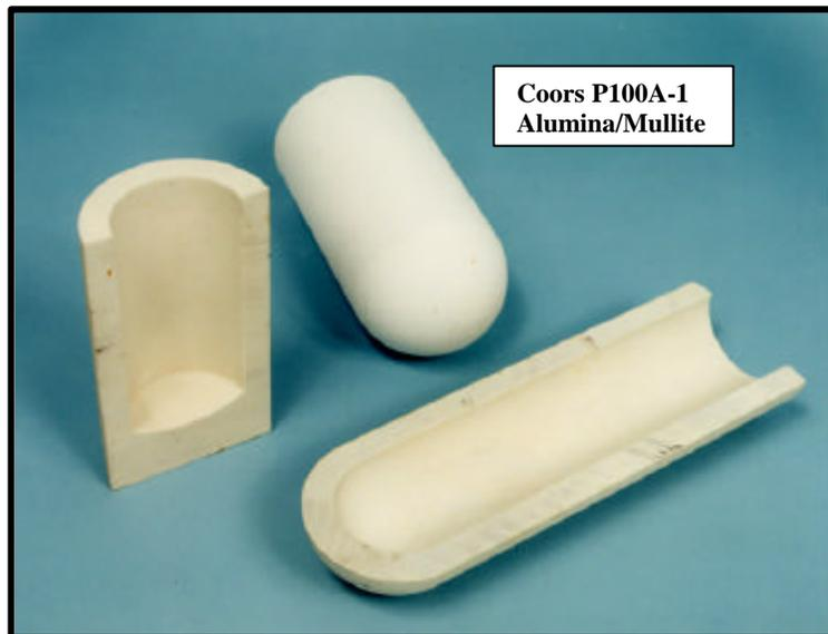
Figure 4 — Variation in the candle filter closed end cap geometry.
