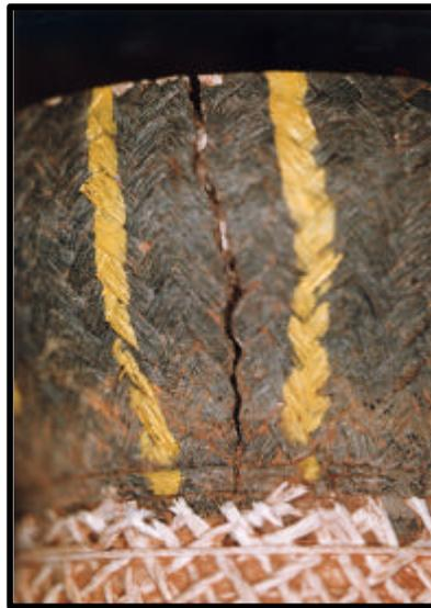
Figure 52 — Failure of the thinner walled 3M CFCC filter element flange.
