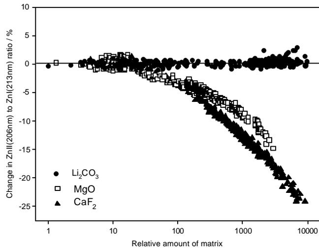
Figure 2. Percentage ratio change of Zn ionic to atomic emission lines in the ICP as a function of a relative amount of  $\text{CaF}_2$ ,  $\text{MgO}$ , and  $\text{Li}_2\text{CO}_3$  matrices.
