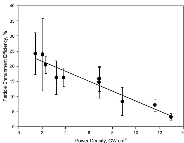
Figure 1: Effect of the laser power density (irradiance) on transport efficiency
