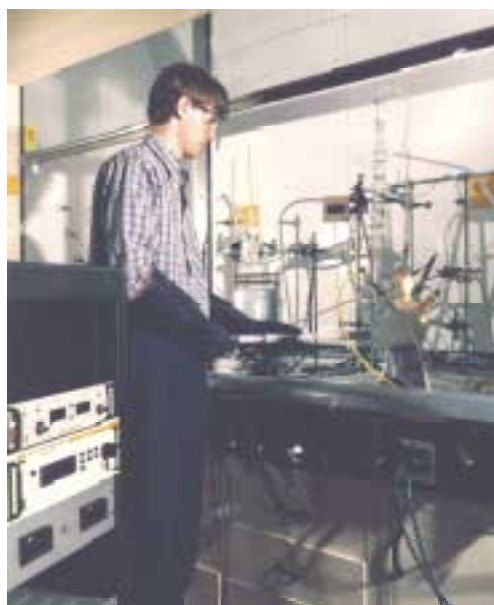
Figure 2. Experimental setup for vapor-liquid-equilibria experiments using electric fields.
