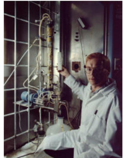
**Figure 2.** ORNL Researcher Thomas Klasson working with one of four trickling biofilter reactors designed to remove dilute organics from contaminated air streams. Reactors were packed with structured packing units, woven out of polyethylene.
