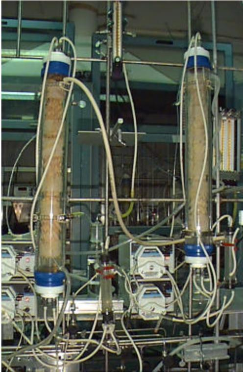
*Figure 1. Two current biotrickling filters from which all biomass analyses were performed. (Photo courtesy*
