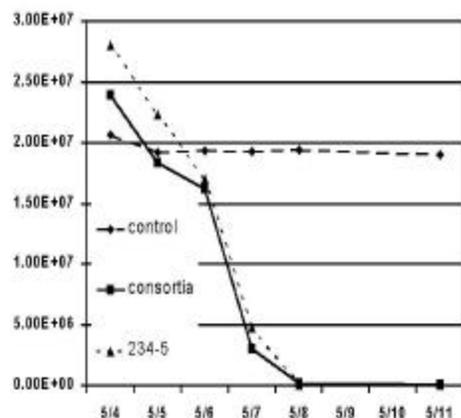
Figure 7. Propane degradation over 7 days.
