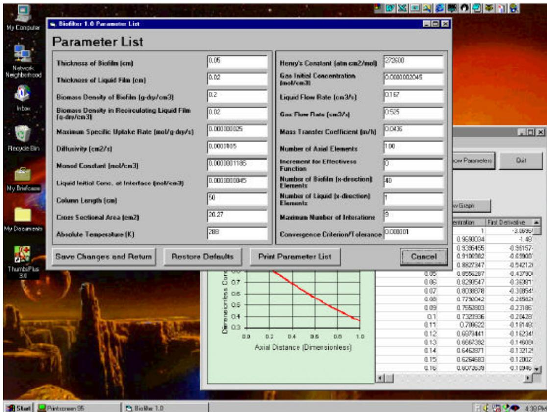
**Figure 5.** Biofilter 1.0 design software was developed for Windows 95/98™ to enable users to quickly and easily determine how various operating parameters will impact their biofilter designs a priori. The user interface is straightforward; data may be copied and then pasted into spreadsheets or presentation packages. Calculation times vary from 1 to 30 seconds on Pentium™-class processors.
