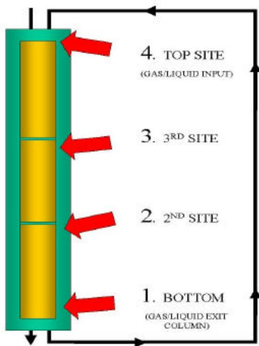
*Figure 3. Simple diagram of the biotrickling filter showing sampling points for population and distribution assay*
