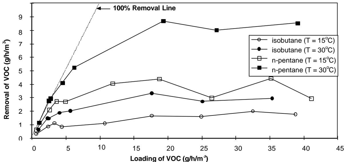
**Figure 3.** Removal Efficiencies in Trickle-bed Bioreactor. Removal efficiencies are highest as the residence time within the trickle-bed system increases. Of the two gases, n-pentane is preferentially removed. The solid line represents 100% removal. Data above were collected for low initial gas phase concentrations in the VOC feed. Higher removal rates are obtained when the initial gas phase concentration is raised.
