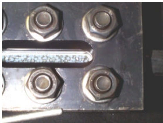
Figure 1. Photoreactor filled with a top layer of TiO 2 coated Pyrex beads and lower layer of uncoated beads.
