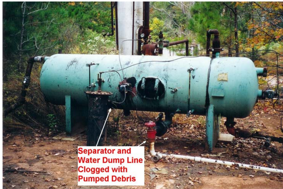
Figure 9. Photograph of 3-phase separator initially used in production.
