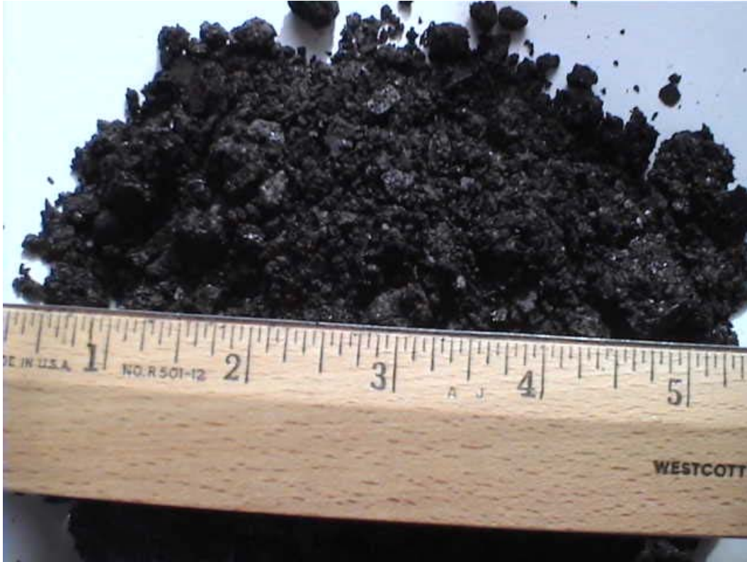
Figure 7. Photograph of debris pumped from wells after treatment.
