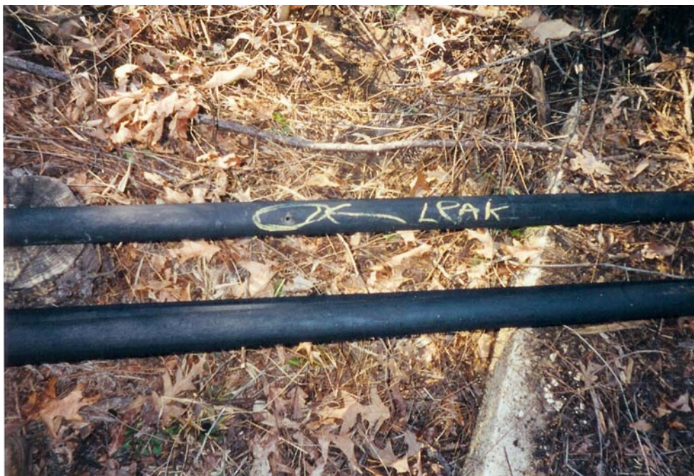
Figure 1. Tubing leak that was discovered post-treatment in the Finney No. 1 well.
