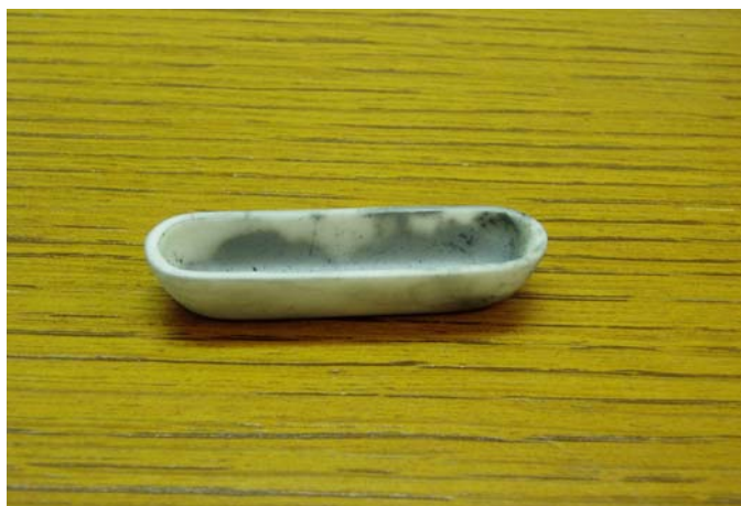
Figure 10. Photograph of combustion boat showing graphite deposits on walls covered by ceria during heating in methane.
